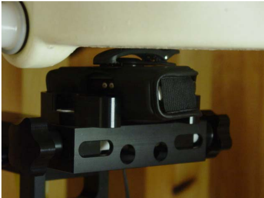
Figure 12.6 body SAR setup (with holster Model: CV90-P096A)
