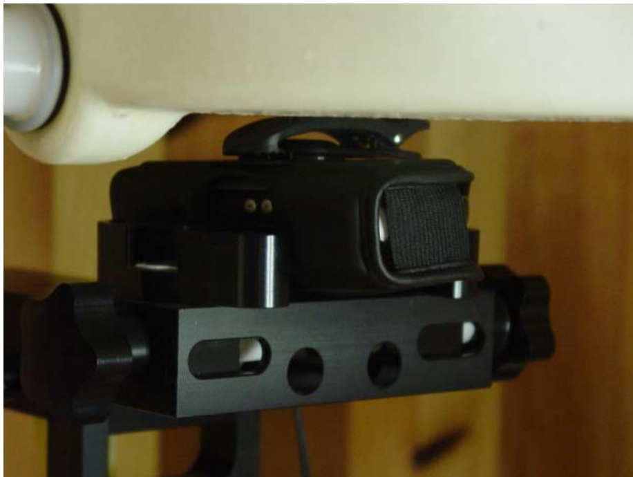
Figure 12.5 body SAR setup (with holster Model: CV90-61346)
