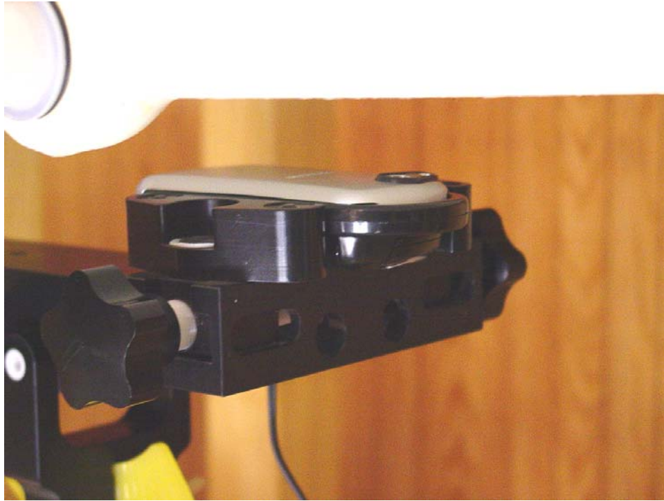
Figure 12.4 body SAR setup (with 25mm air separation)
