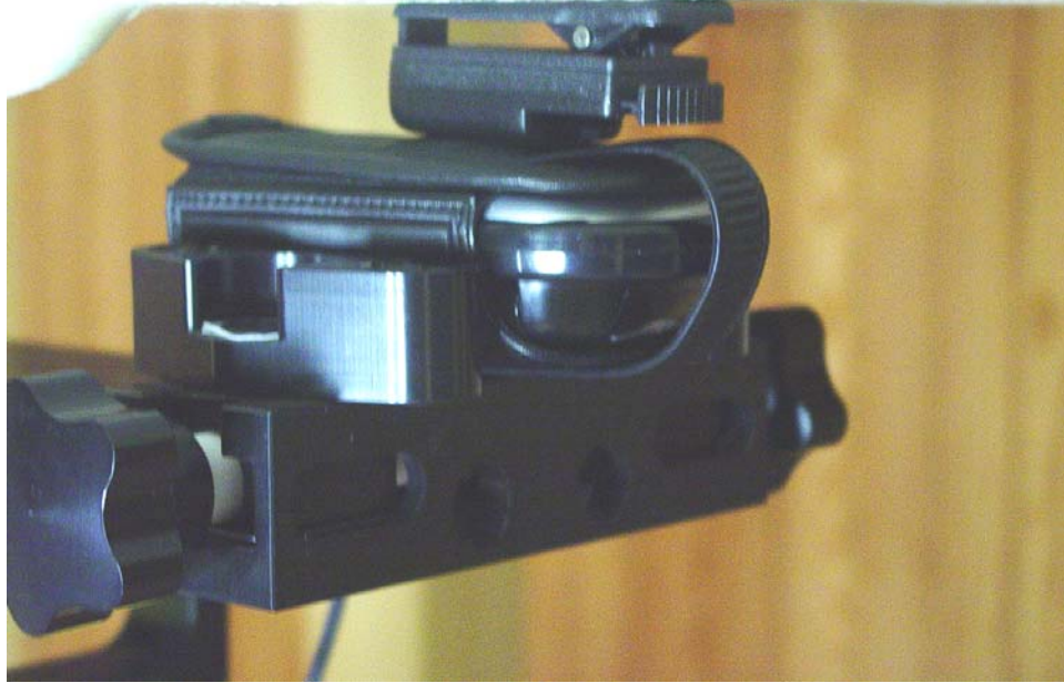
Figure 12.5 body SAR setup (with holster Model: CV90-61346)
