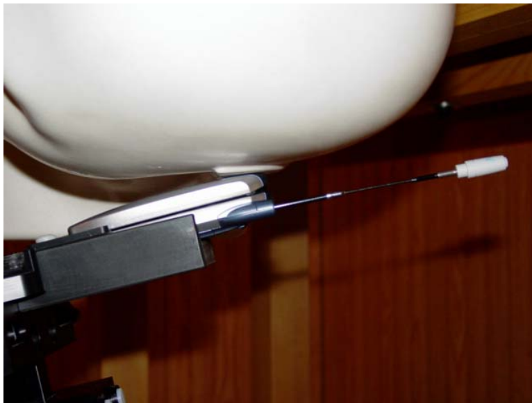
Figure 10.5 phone against the head (right tilt position, swivel closed, antenna extended)
