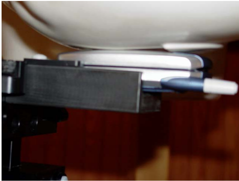
Figure 10.2 phone against the head (right cheek position, swivel closed, antenna retracted)
