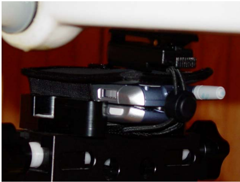
Figure 10.12 body SAR setup (with leather case, swivel closed, antenna retracted)
