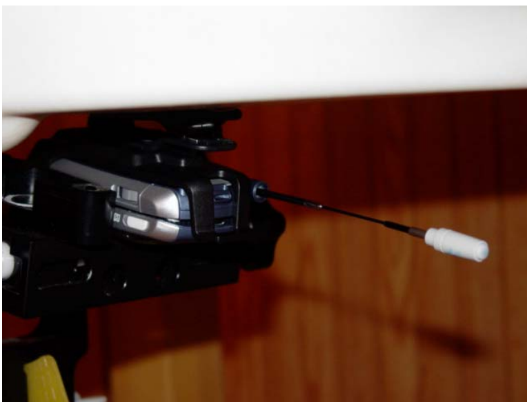
Figure 10.11 body SAR setup (with holster, swivel closed, antenna extended)
