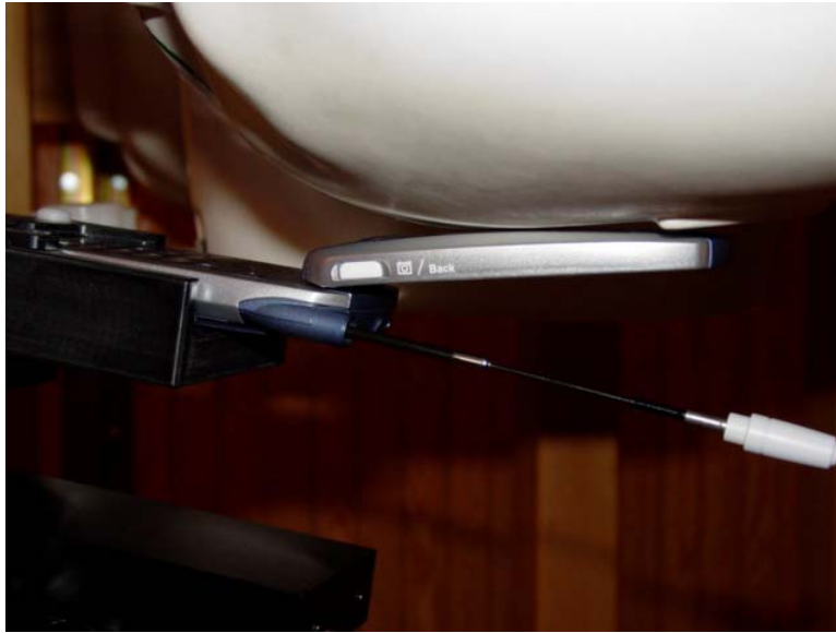
Figure 10.8 phone against the head (right cheek position, swivel open, antenna extended)
