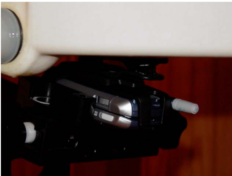
Figure 10.10 body SAR setup (with holster, swivel closed, antenna retracted)
