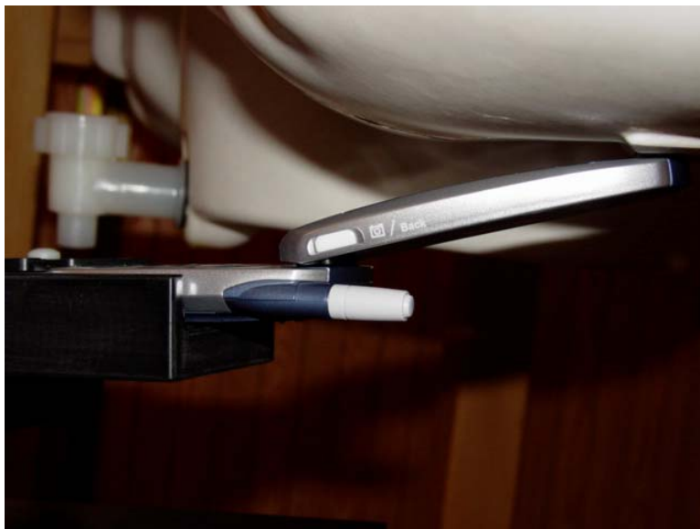
Figure 10.7 phone against the head (right tilt position, swivel open, antenna retracted)
