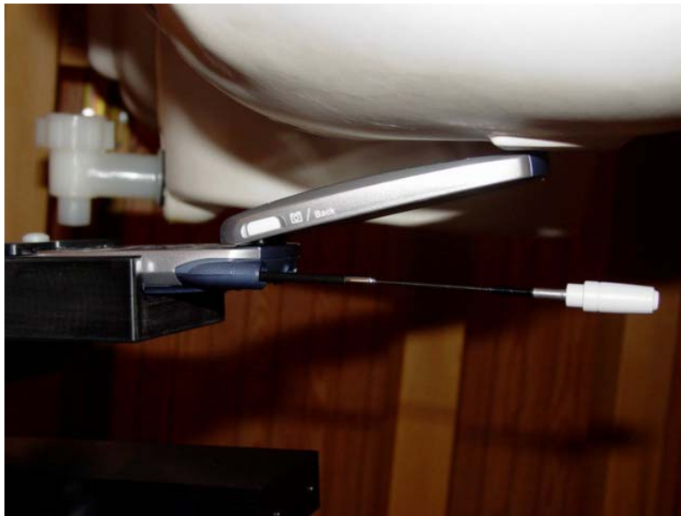
Figure 10.9 phone against the head (right tilt position, swivel open, antenna extended)
