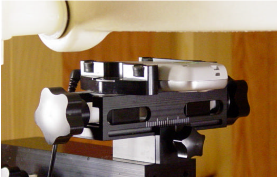
Figure 10.6 Body SAR Set-up (with 25mm air separation)
