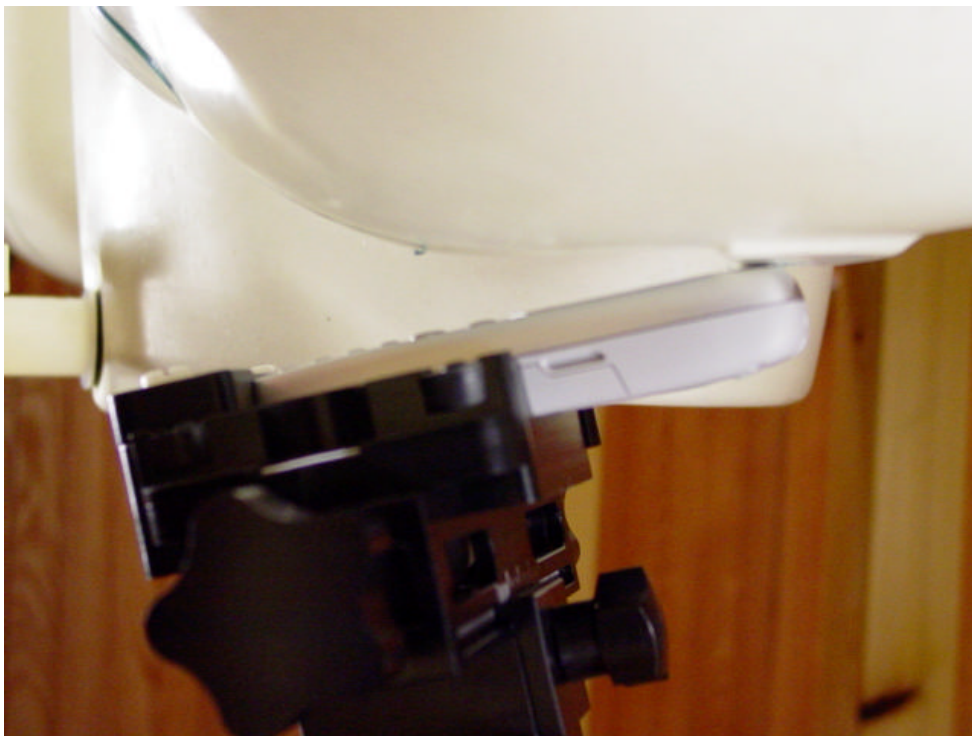
Figure 12.3 phone against the head (left tilt position)
