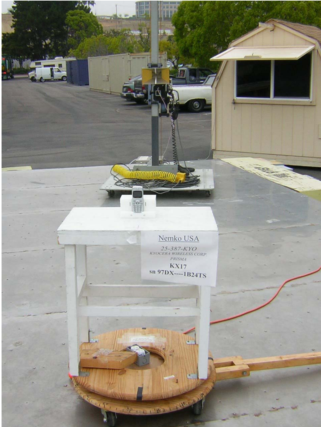
Photograph 1. FCC, Part 22 Radiated Emissions Test Configuration
