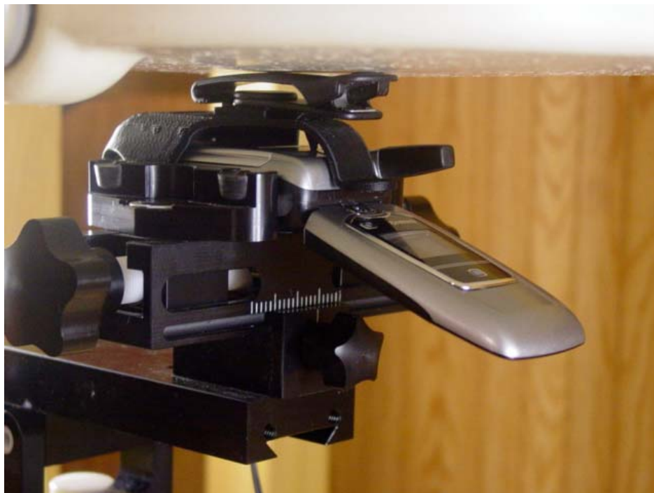
Figure 12.4 body SAR setup open (with holster)
