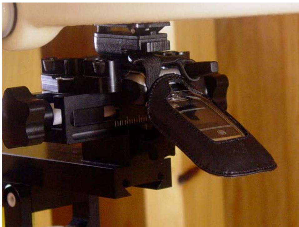
Figure 12.7 body SAR setup open (with leather case)
