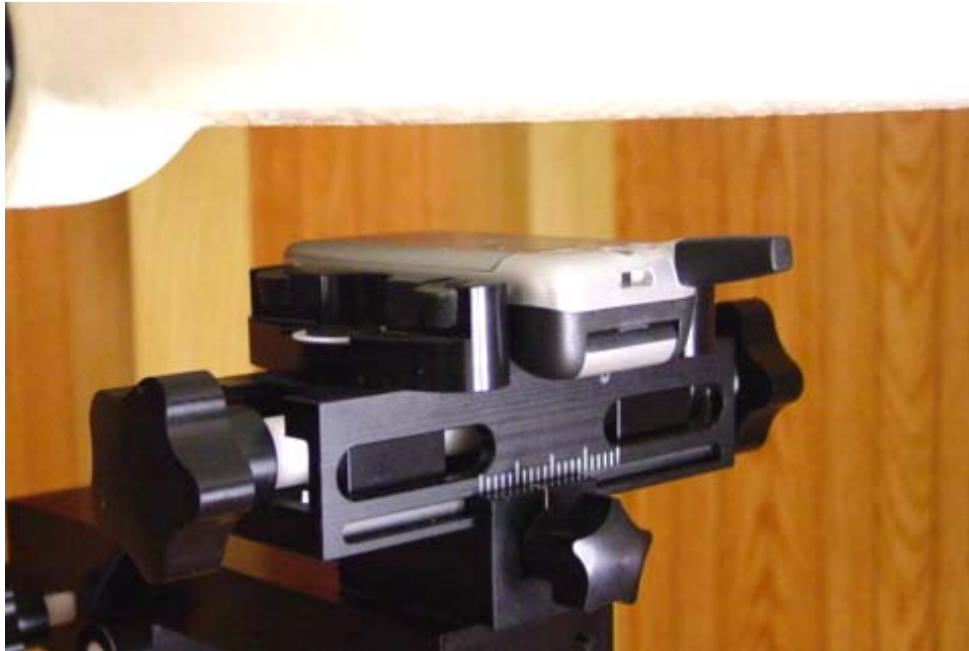
Figure 12.5 body SAR setup closed (with 25mm air separation)
