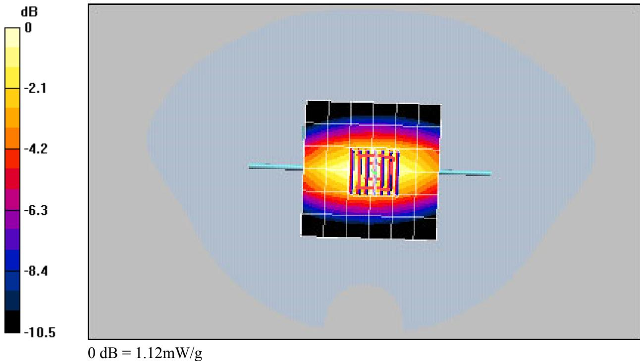
**FCC 1900MHz Validation@20.00dBm, Probe#1713, DAE#602, Dipole#5d005****Communication System: CW 1900, Frequency: 1900 MHz, Duty Cycle: 1:1****Medium: HSL1800, Medium parameters used (interpolated):  $f = 1900 \text{ MHz}$ ;  $\sigma = 1.39 \text{ mho/m}$ ;  $\epsilon_r = 41.5$ ;  $\rho = 1000 \text{ kg/m}^3$** **Phantom: SAM 12, Phantom section: Flat Section****DASY4 Configuration:**
