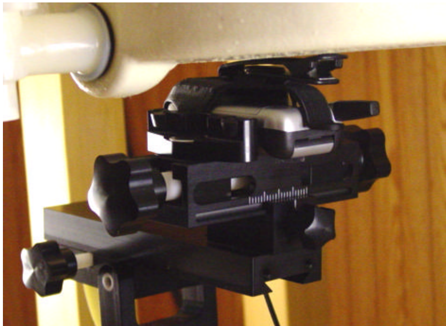
Figure 12.3 body SAR setup closed (with holster)
