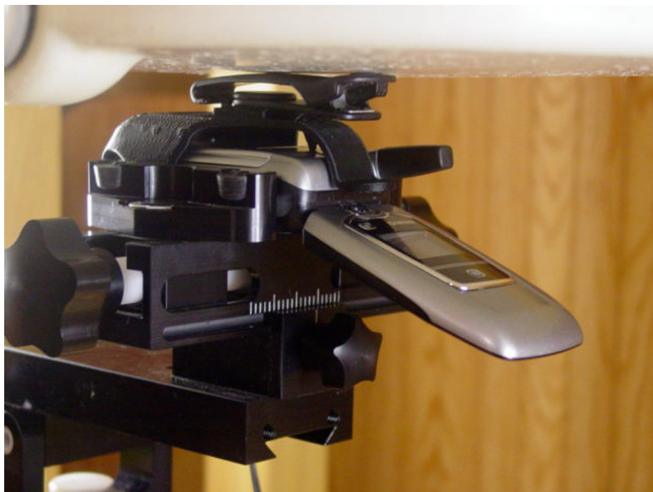
Figure 12.4 body SAR setup open (with holster)
