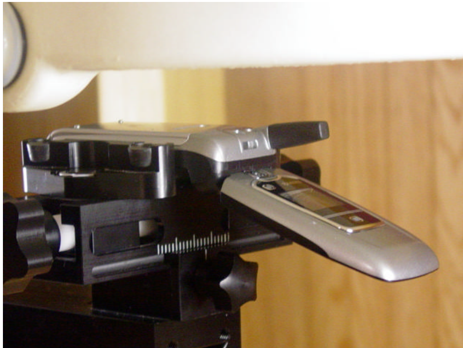
Figure 12.6 body SAR setup open (with 25mm air separation)
