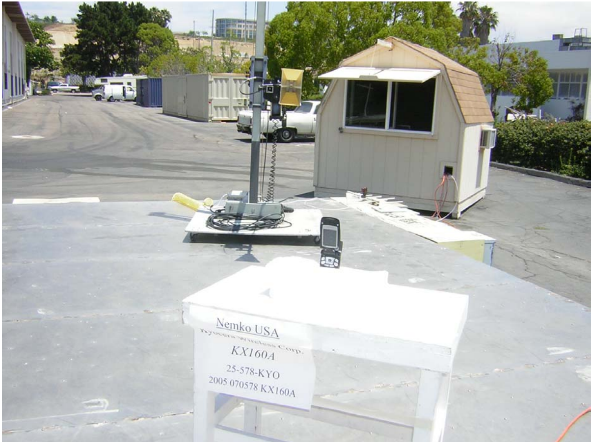
Photograph 3. FCC, Part 22/24 Radiated Emissions Test Configuration
