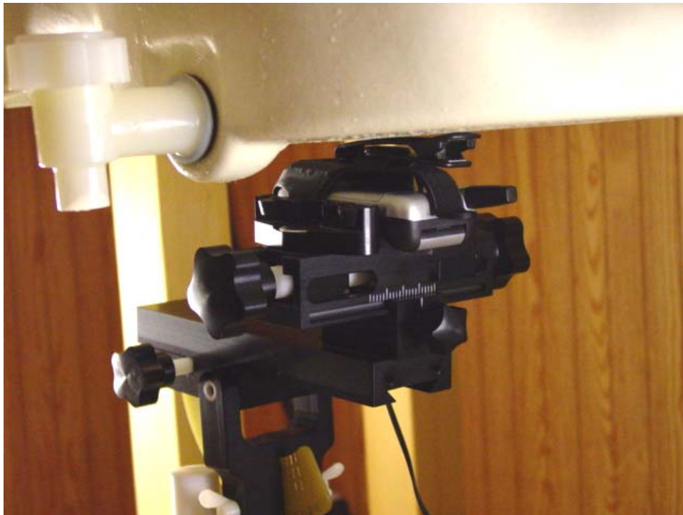
Figure 12.3 body SAR setup closed (with holster)
