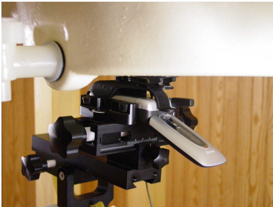
Figure 12.4 body SAR setup open (with holster)
