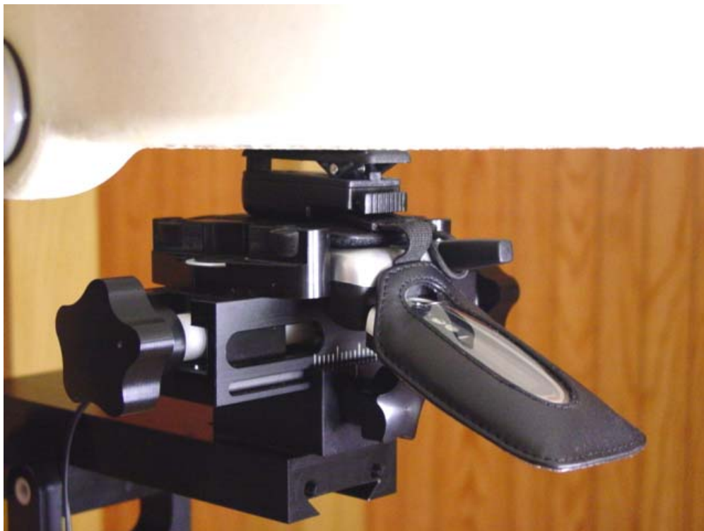
Figure 12.7 body SAR setup open (with leather case)
