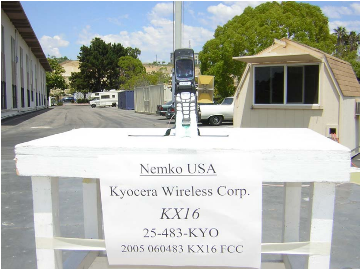
Photograph 3. FCC, Part 22/24 Radiated Emissions Test Configuration
