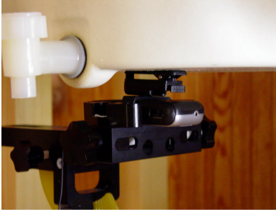
Figure 12.4 body SAR setup (with holster)
