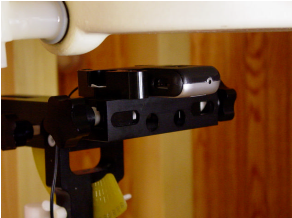
Figure 12.5 body SAR setup (with 25mm air separation)
