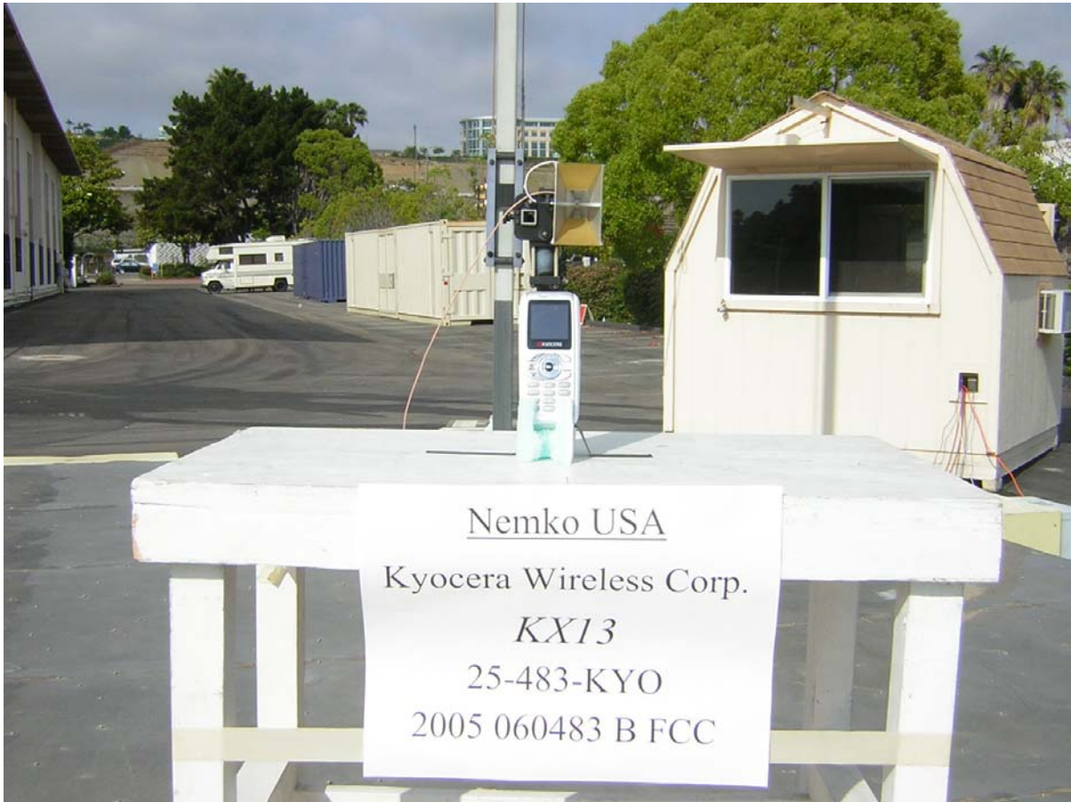
Photograph 3. FCC, Part 22/24 Radiated Emissions Test Configuration
