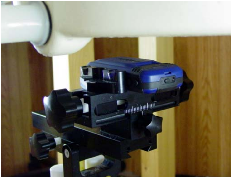
Figure 12.4 body SAR setup (with 25mm air separation)
