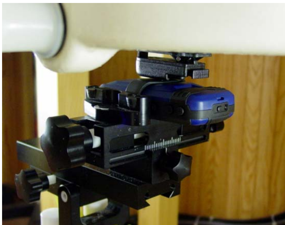
Figure 12.4 body SAR setup (with 25mm air separation)
