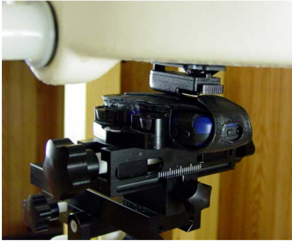
Figure 12.6 body SAR setup (with leather case)
