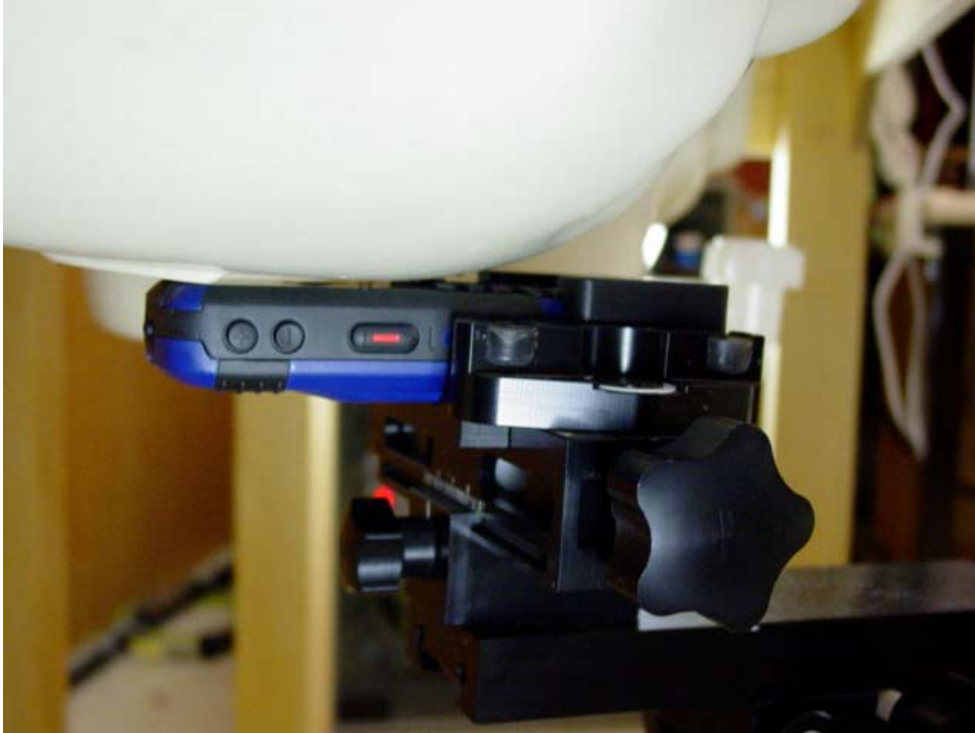
Figure 12.2 phone against the head (right cheek position)
