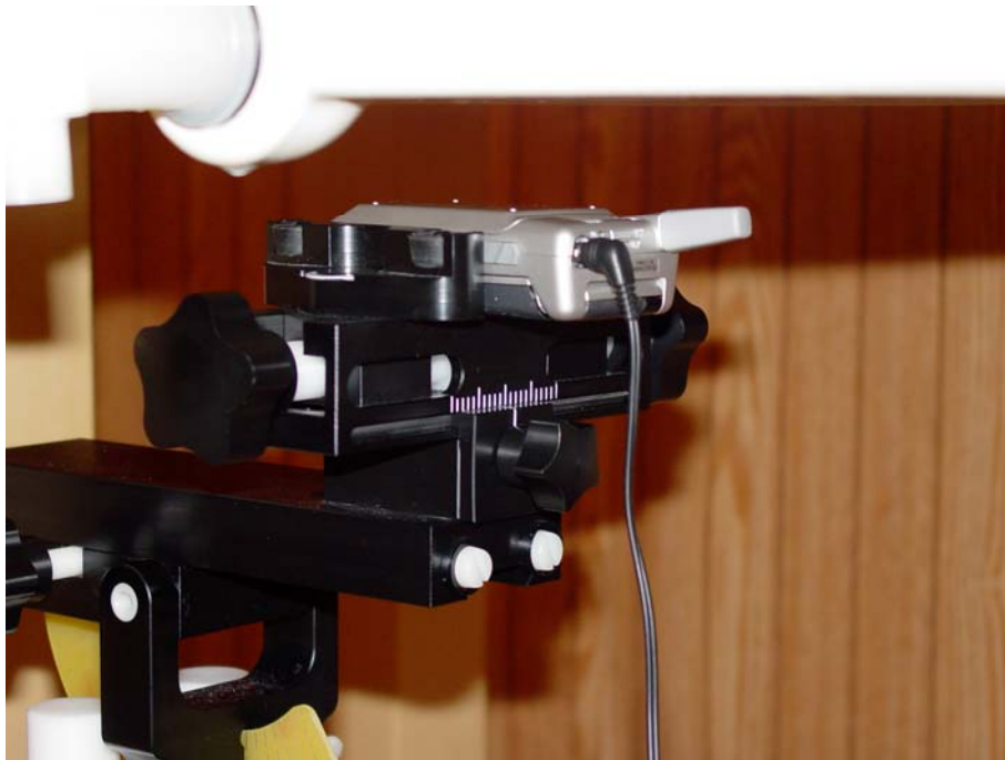
Figure 10.6 body SAR setup (with 25mm air separation)
