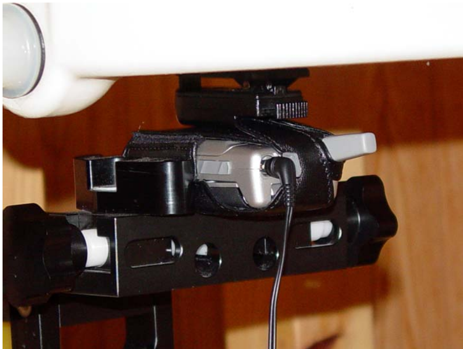
Figure 10.5 body SAR setup (with leather case)
