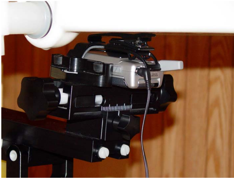
Figure 10.4 body SAR setup (with holster)
