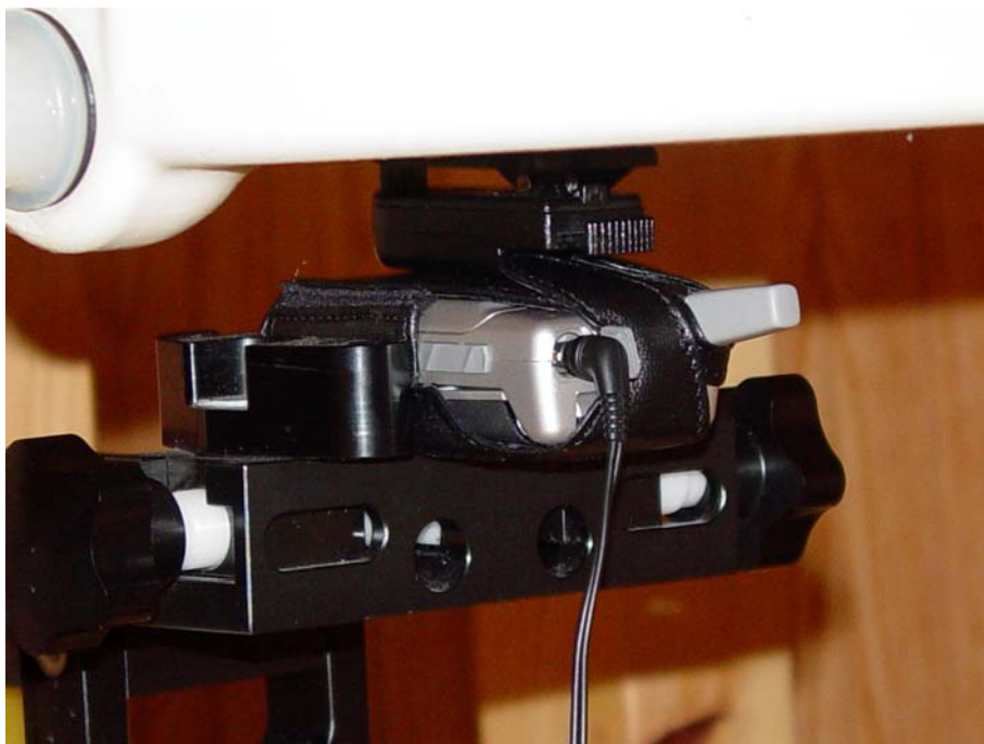
Figure 10.5 body SAR setup (with leather case)
