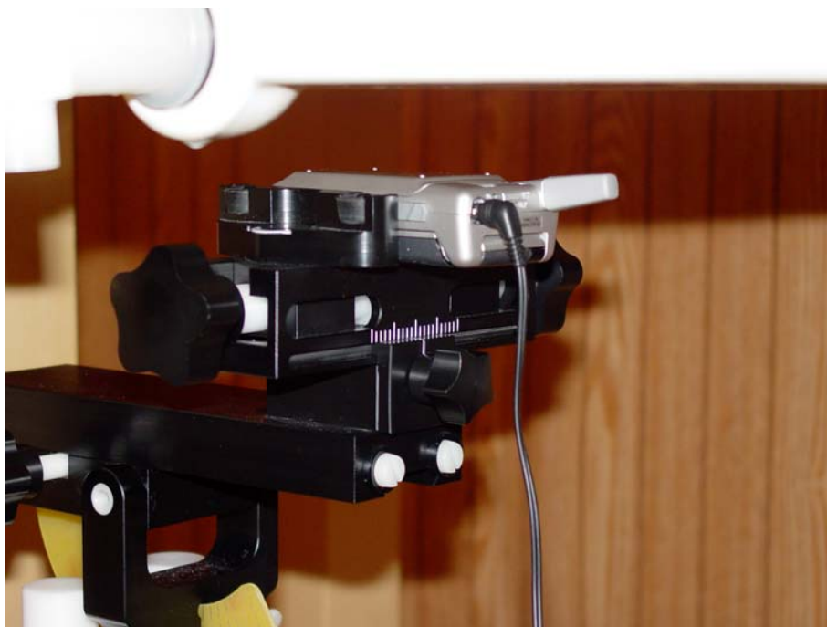
Figure 10.6 body SAR setup (with 25mm air separation)
