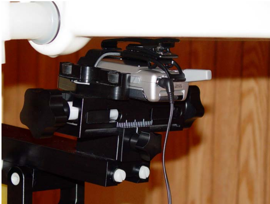
Figure 10.4 body SAR setup (with holster)
