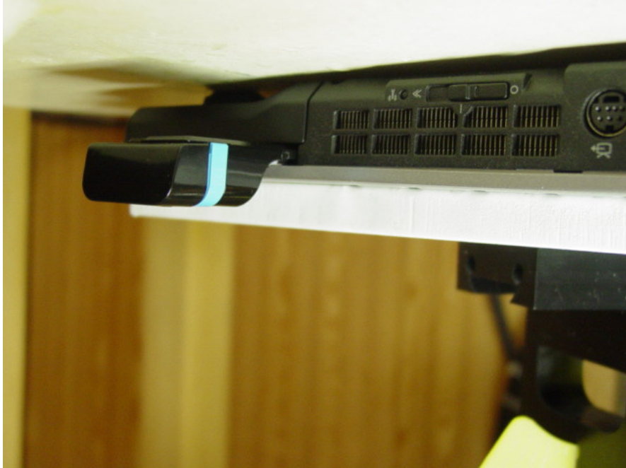
Figure 9E.1 Host Computer #1 against the body (Antenna 0 Degree position)
