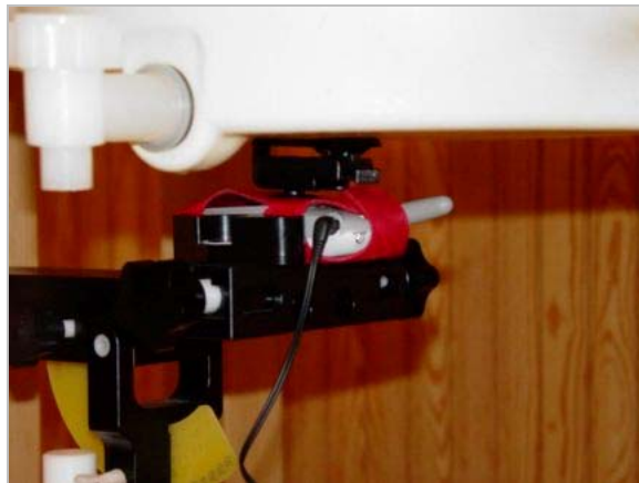
Figure 10.5 body SAR setup (with leather case)
