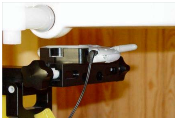
Figure 10.6 body SAR setup (with 22.5mm air separation)
