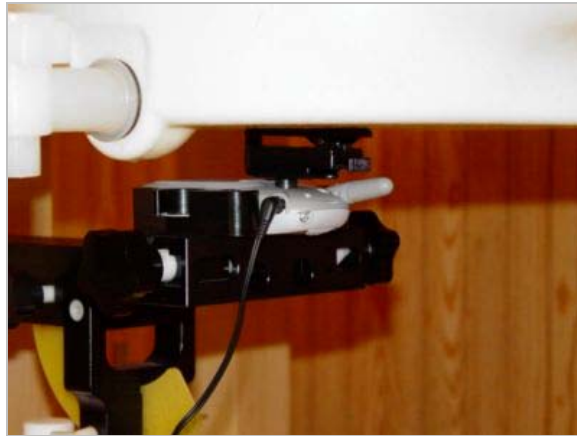
Figure 10.4 body SAR setup (with belt clip)
