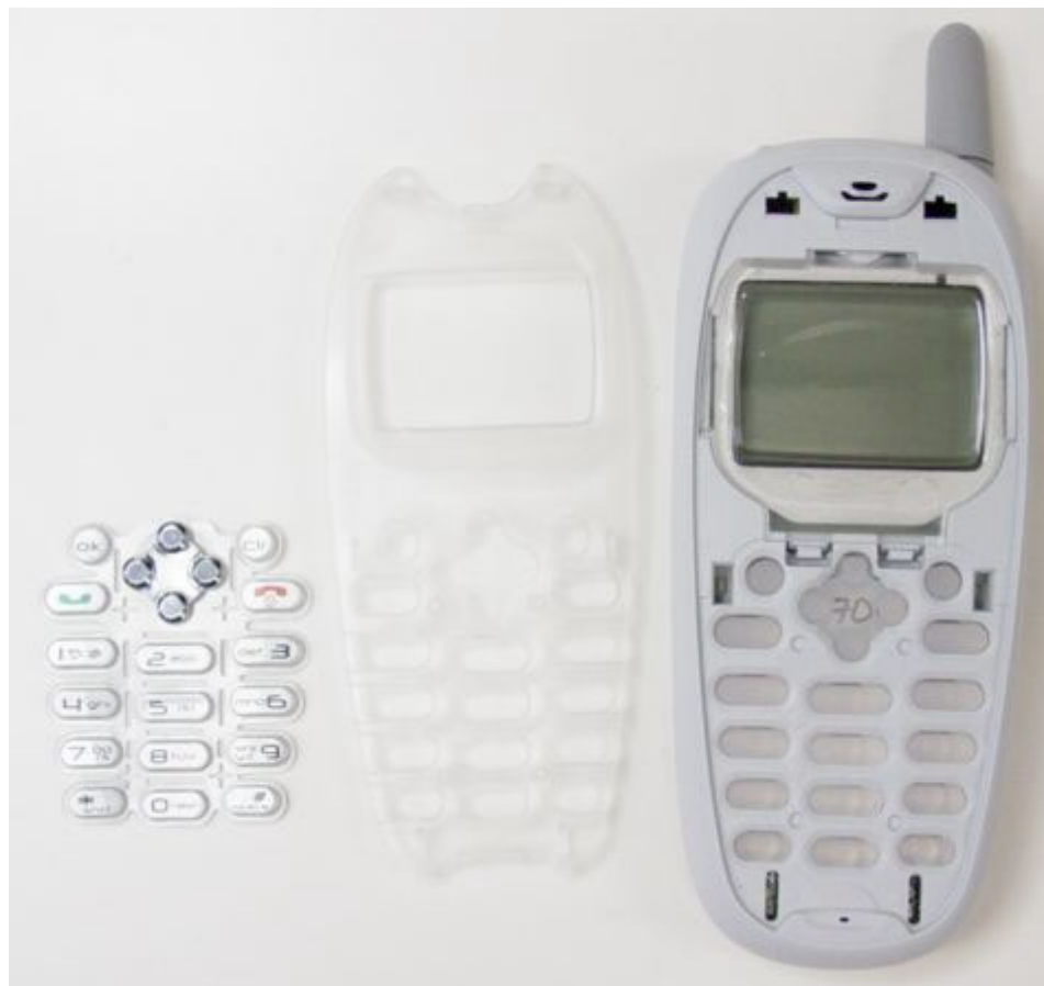
Front Housing with face plate off
