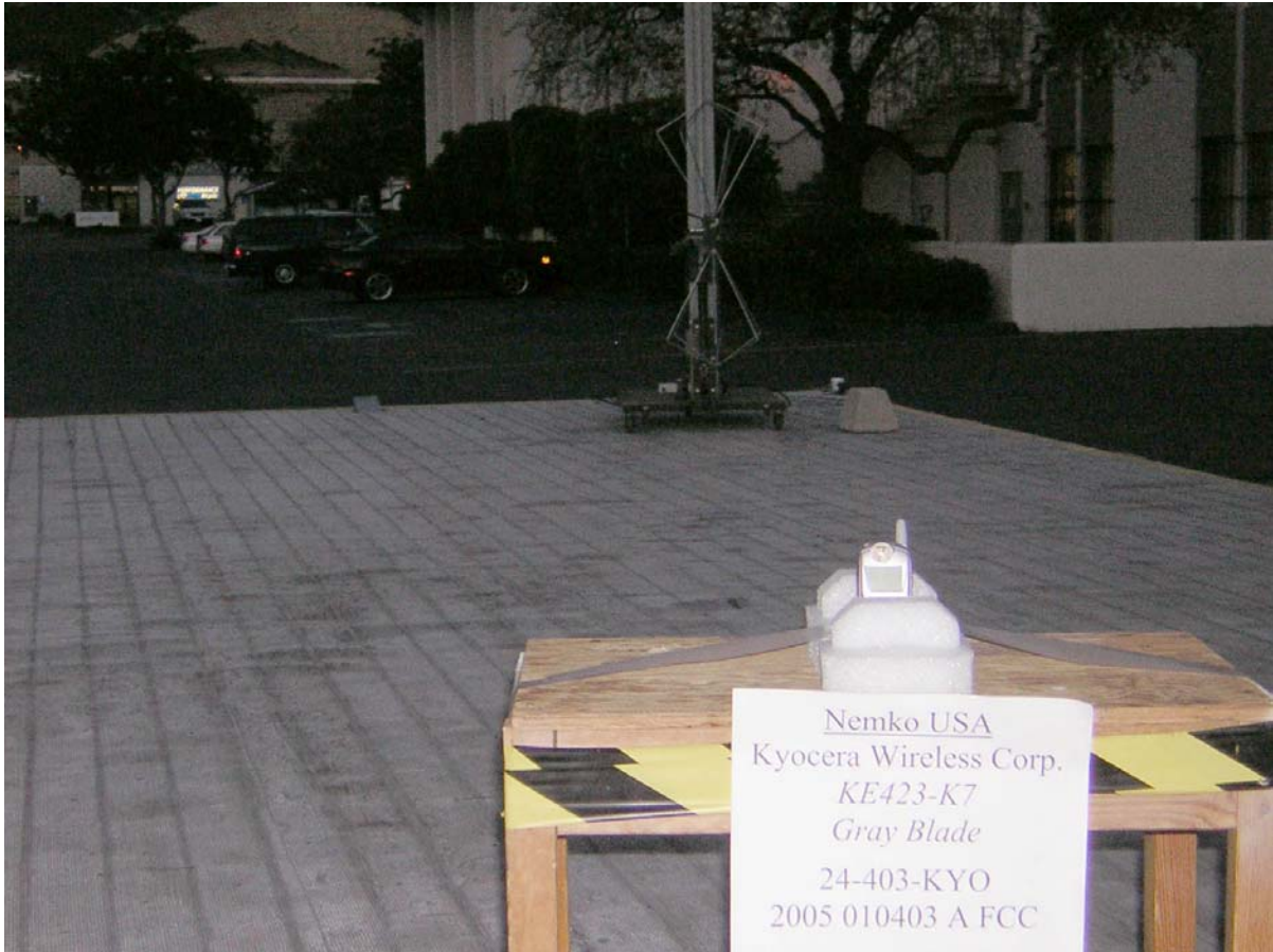
Photograph 2. FCC, Part 15 Radiated Emissions Test Configuration
