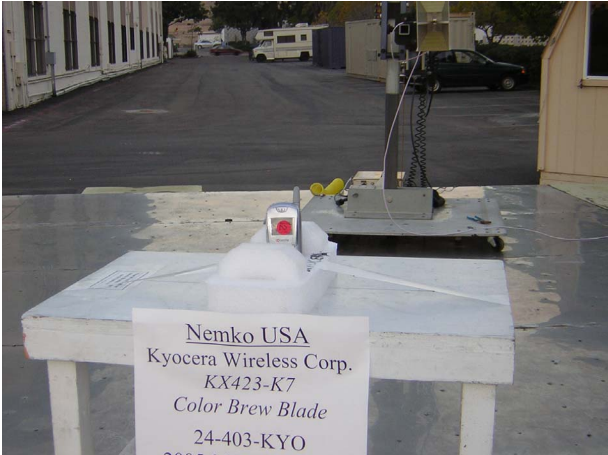
Photograph 1. FCC, Part 24 Radiated Emissions Test Configuration
