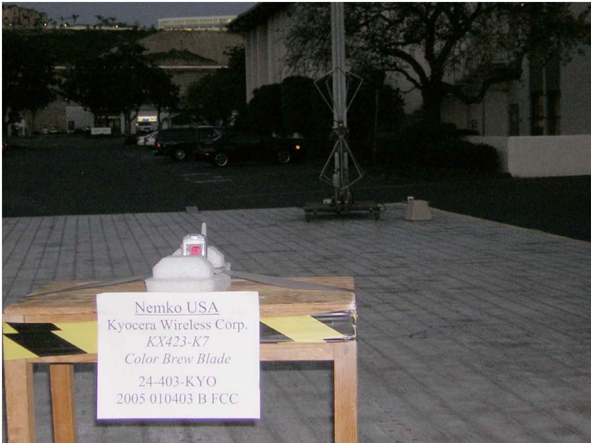
Photograph 2. FCC, Part 15 Radiated Emissions Test Configuration
