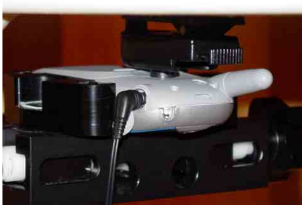
Figure 11.4 body SAR set-up (with belt clip)
