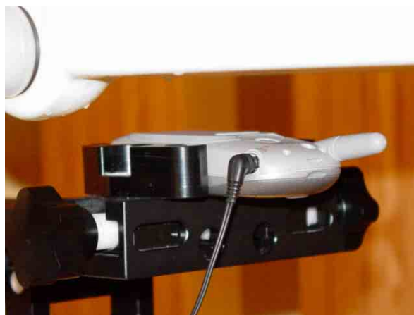
Figure 11.6 body SAR set-up (with 22.5mm air separation)
