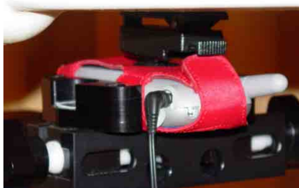
Figure 11.5 body SAR set-up (with leather case)
