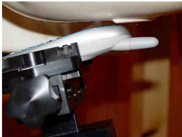
Figure 11.3 phone against the head (left tilt position)
