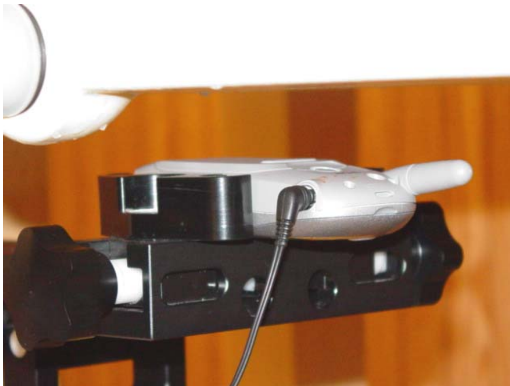
Figure 11.6 body SAR setup (with 22.5 mm air separation)
