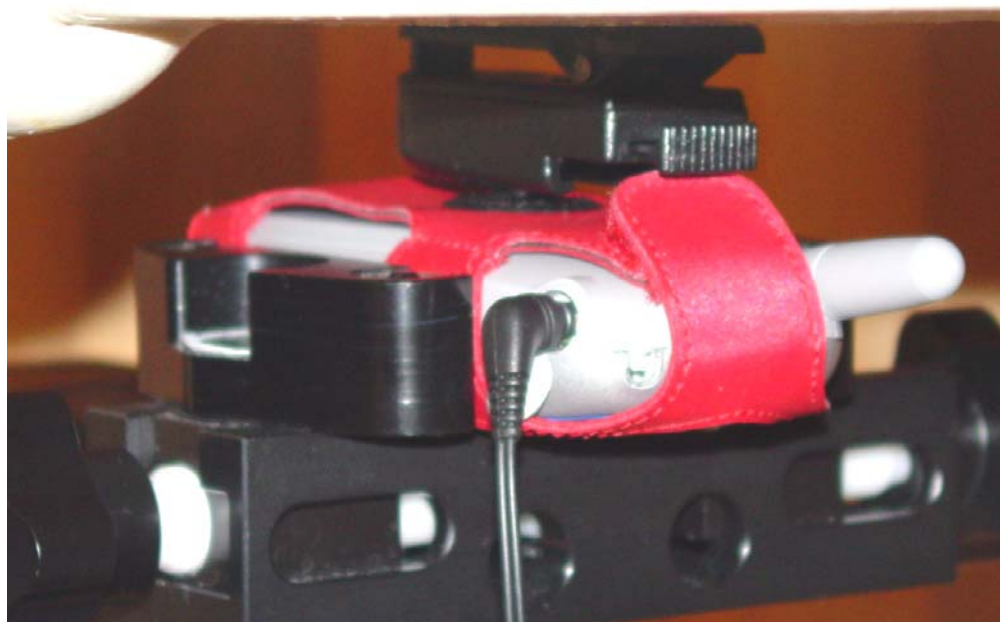
Figure 11.5 body SAR setup (with leather case)
