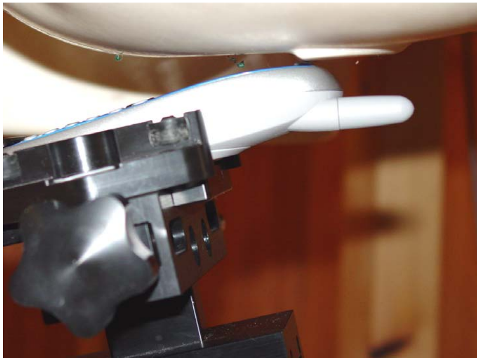
Figure 11.3 phone against the head (left tilt position)
