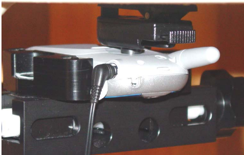
Figure 11.4 body SAR setup (with belt clip)
