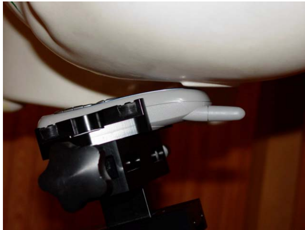
Figure 11.3 phone against the head (left tilt position)
