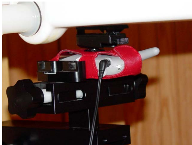
Figure 11.5 body SAR set-up (with leather case)
