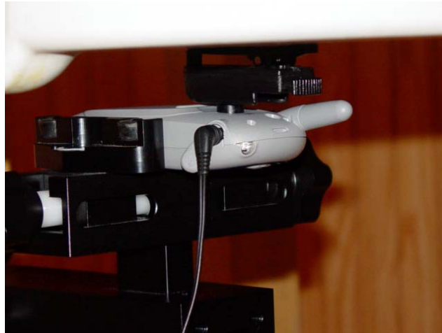
Figure 11.4 body SAR set-up (with belt clip)
