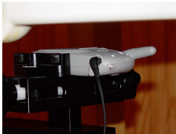
Figure 11.6 body SAR set-up (with 22.5mm air separation)
