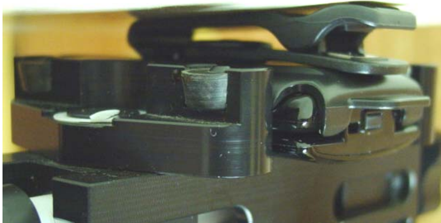
Figure 9E.1 Body SAR setup (CE90-M2595-01 Phone Closed)
