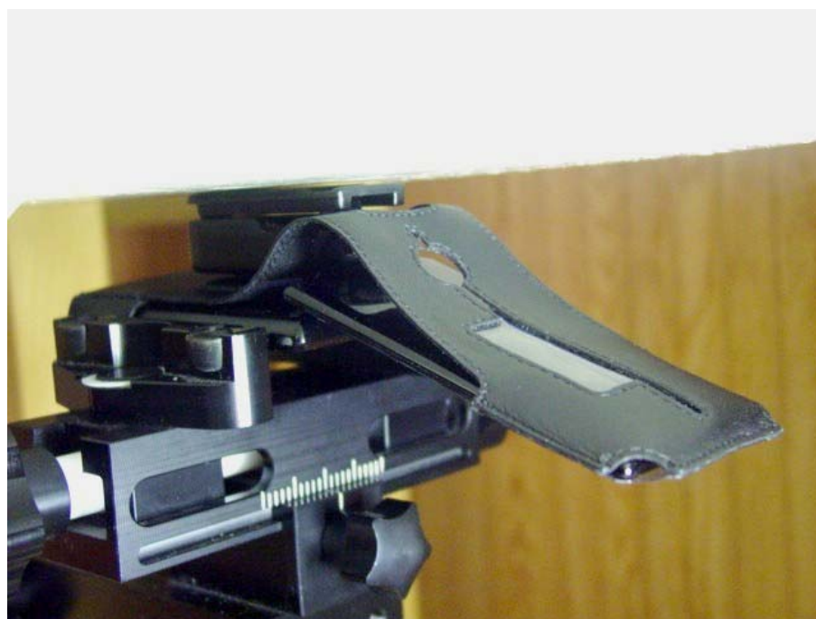
Figure 9E.6 Body SAR setup (CV90-B3916-02 Phone Open)
