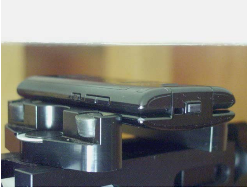
Figure 9E.3 Body SAR setup (15mm Air Separation Phone Closed)
