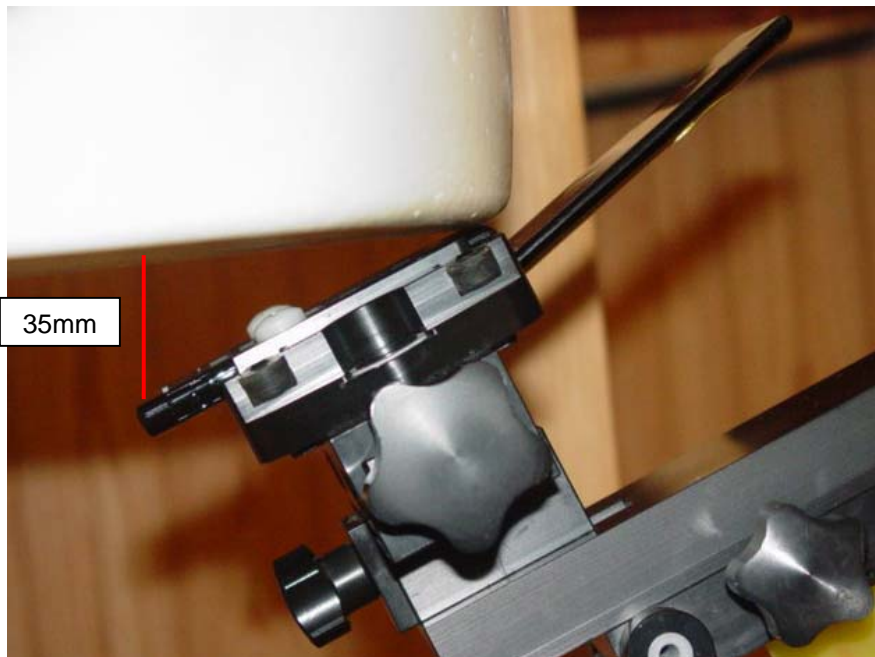
Figure 9E.7 Phone against flat phantom (mouth, jaw position)
