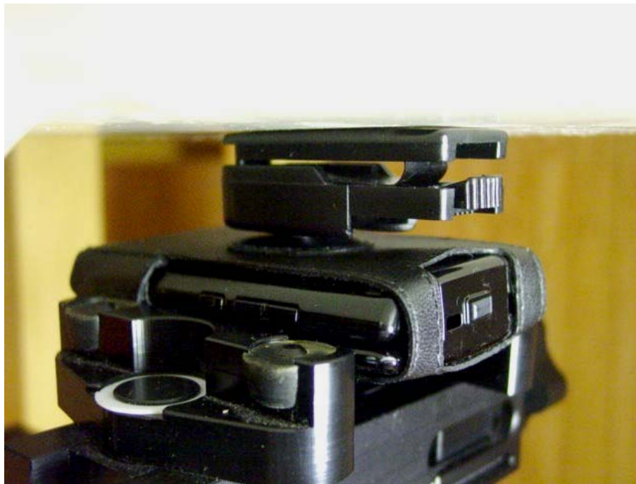
Figure 9E.5 Body SAR setup (CV90-B3916-02 Phone Closed)
