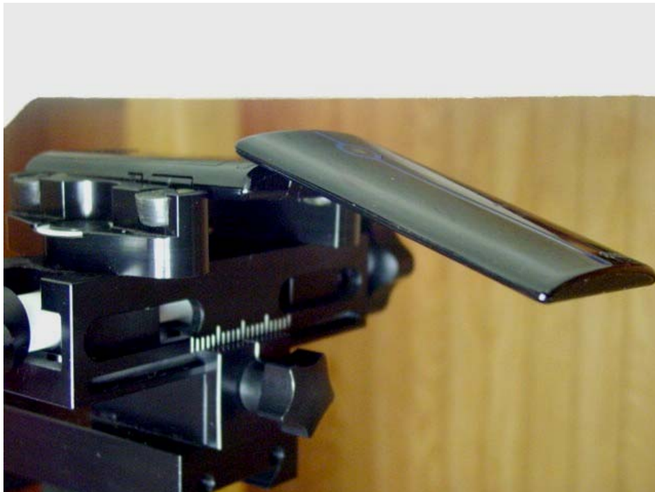
Figure 9E.4 Body SAR setup (15mm Air Separation Phone Open)
