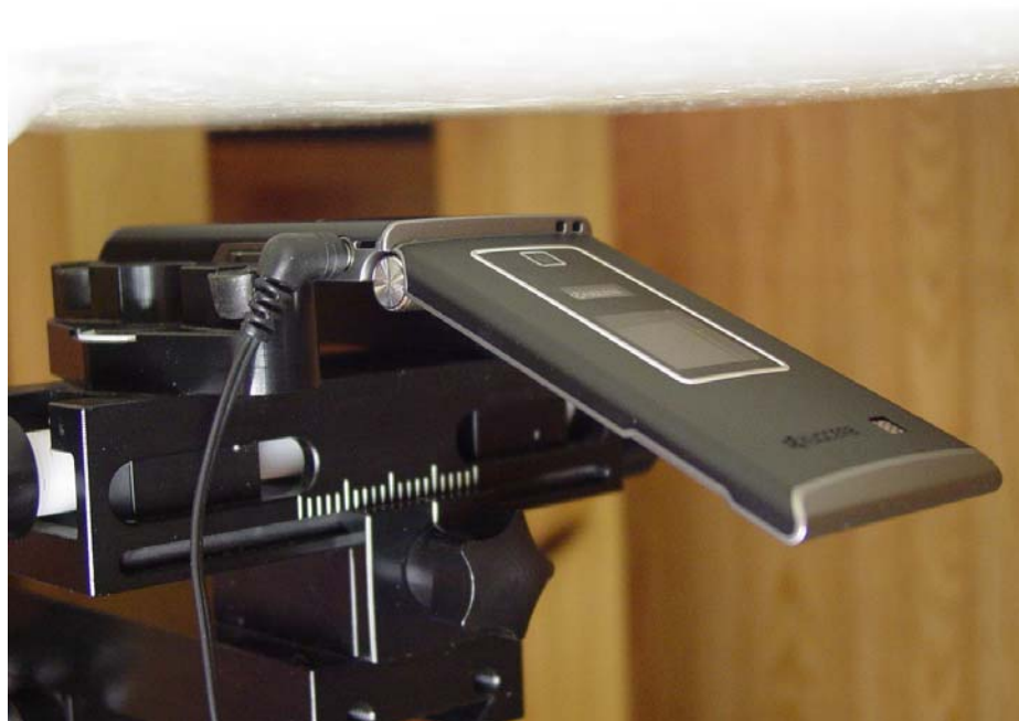
Figure 9E.4 Body SAR setup (15mm Air Separation Phone Open)
