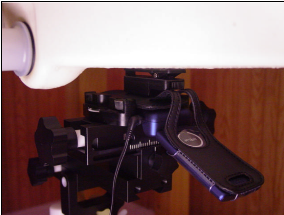
Figure 9E.6 body SAR setup open (with standard case)
