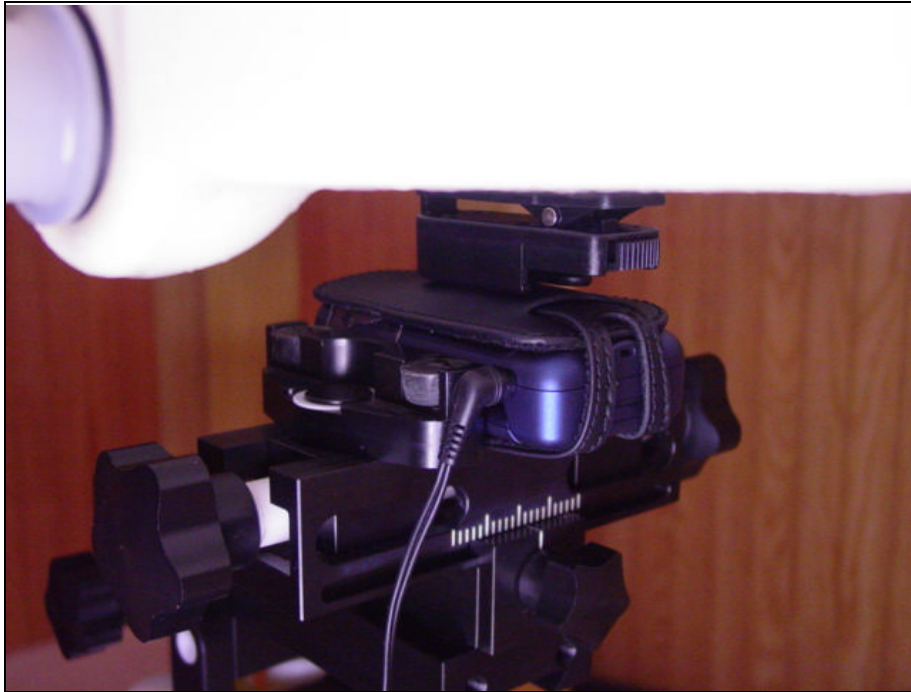
Figure 9E.5 body SAR setup closed (with standard case)
