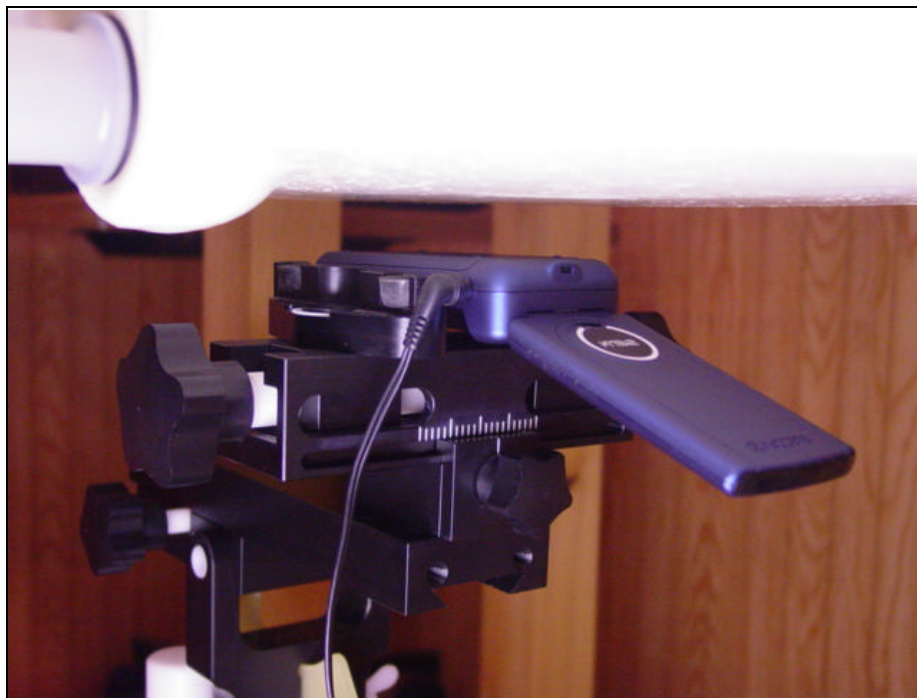
Figure 9E.4 body SAR setup open (with 15mm air separation)
