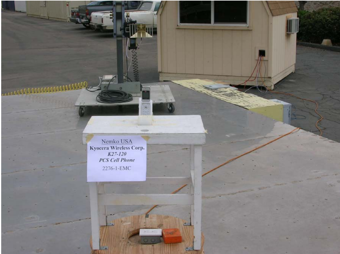
Figure 4. FCC, Part 24 Radiated Emissions Test Configuration
