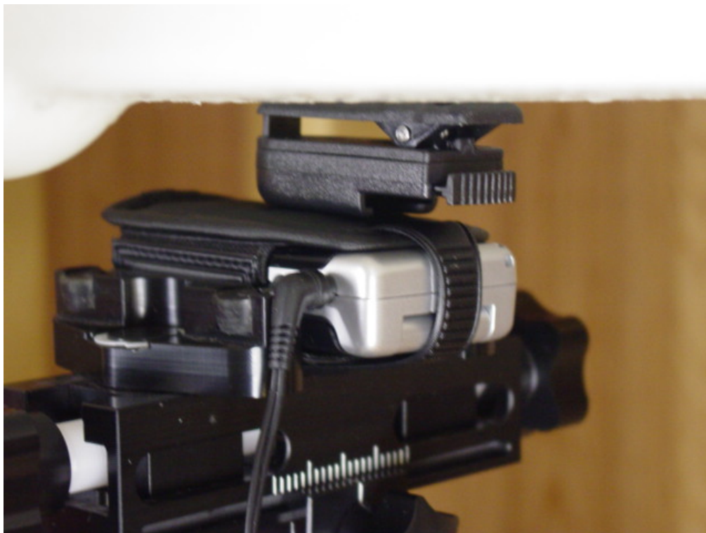
Figure 9E.5 Body SAR setup phone closed (with CV90-M2834-01)
