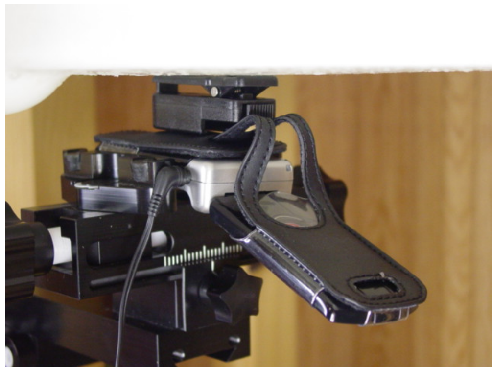
Figure 9E.6 Body SAR setup phone open (with CV90-M2834-01)
