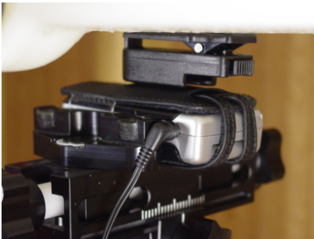
Figure 9E.7 Body SAR setup phone closed (with CV90-61345-03)
