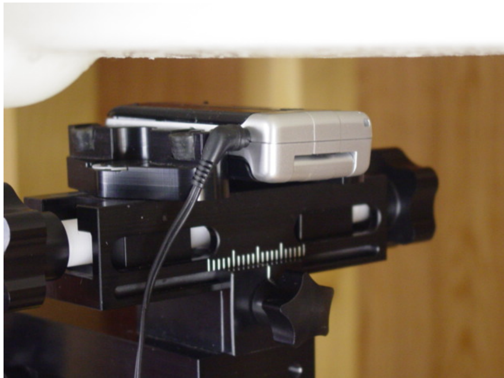
Figure 9E.3 Body SAR setup phone closed (with 15mm air separation)
