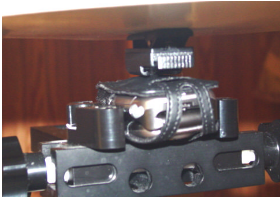
Figure 9E.5 body SAR setup closed (with standard case)
