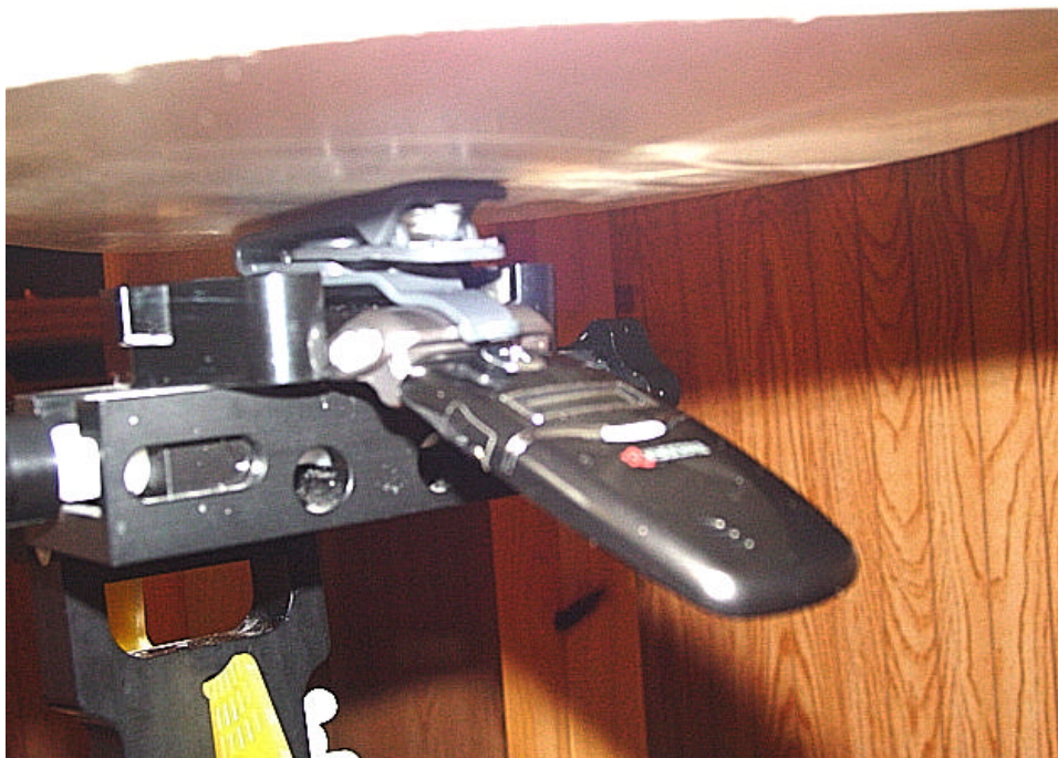
Figure 9E.8 body SAR setup open (with Holster)
