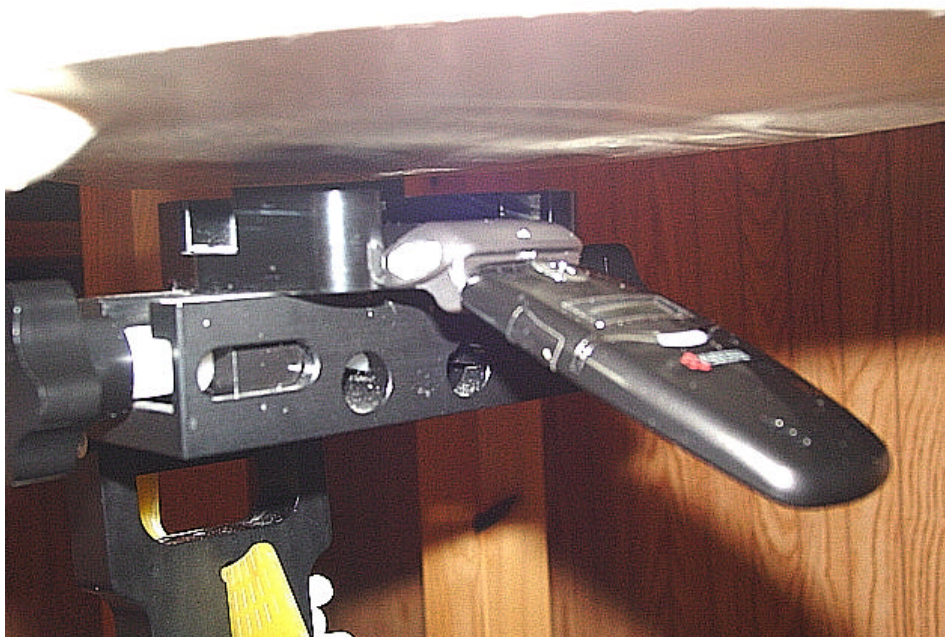
Figure 9E.4 body SAR setup open (with 15mm air separation)
