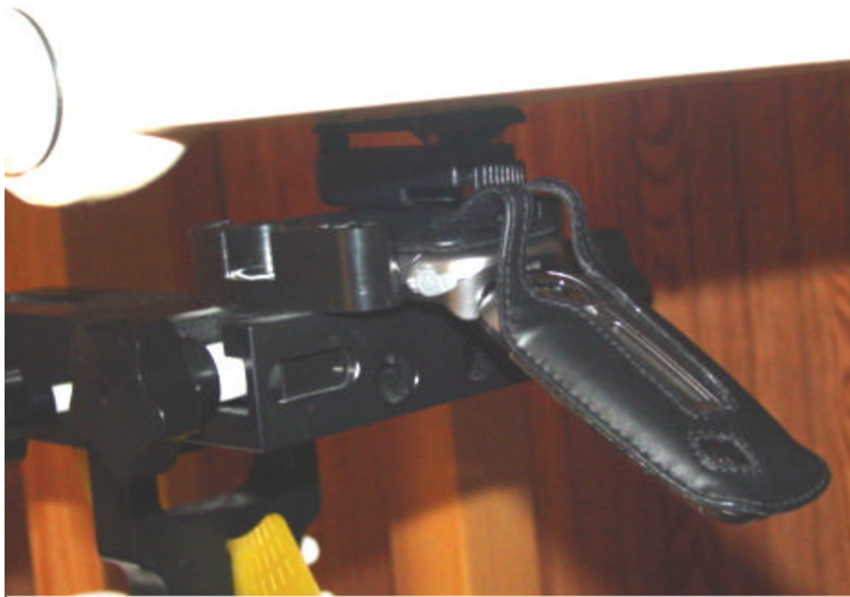
Figure 9E.6 body SAR setup open (with standard case)
