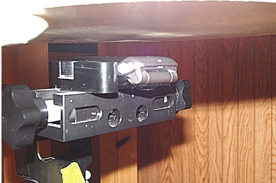
Figure 9E.3 body SAR setup closed (with 15mm air separation)
