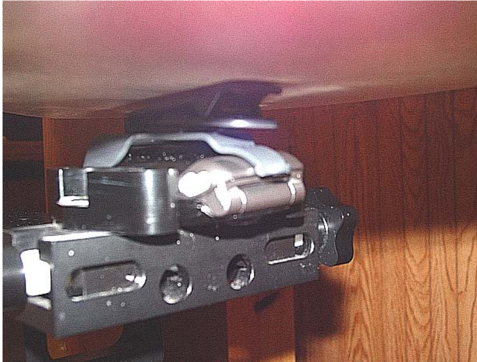
Figure 12.3 body SAR setup closed (with holster)
