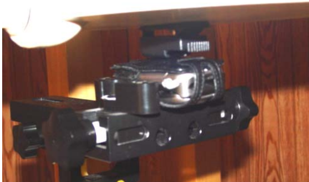
Figure 12.9 body SAR setup closed (with premium case)
