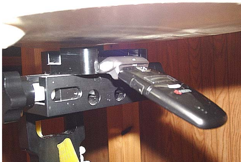
Figure 12.6 body SAR setup open (with 15mm air separation)
