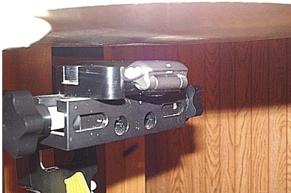
Figure 12.5 body SAR setup closed (with 15mm air separation)
