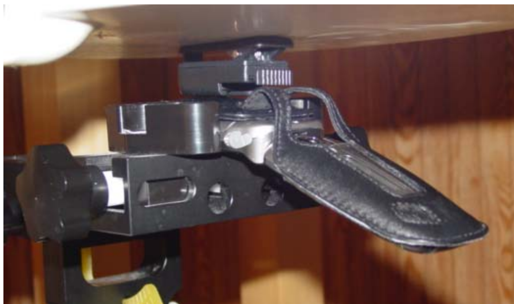
Figure 12.9 body SAR setup open (with premium case)
