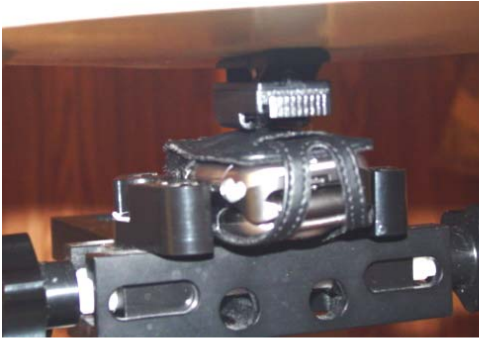
Figure 12.7 body SAR setup closed (with standard case)
