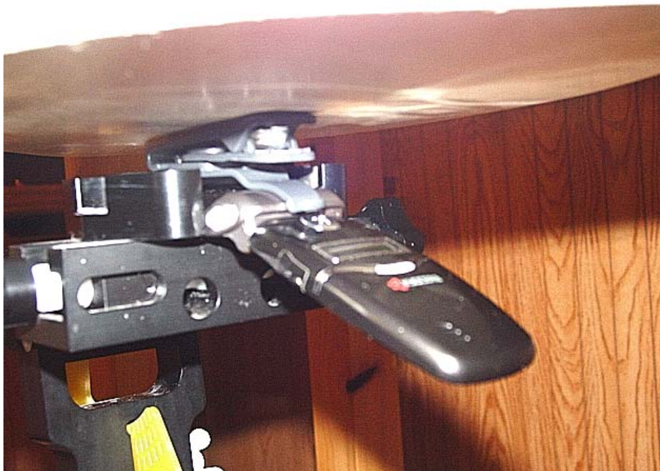
Figure 12.4 body SAR setup open (with holster)
