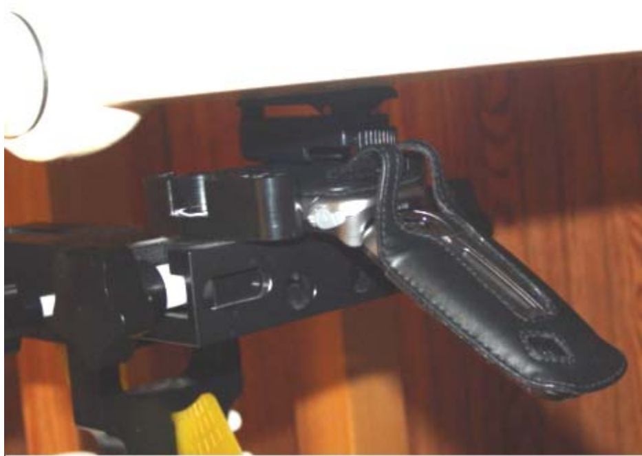
Figure 12.9 body SAR setup open (with standard leather case)
