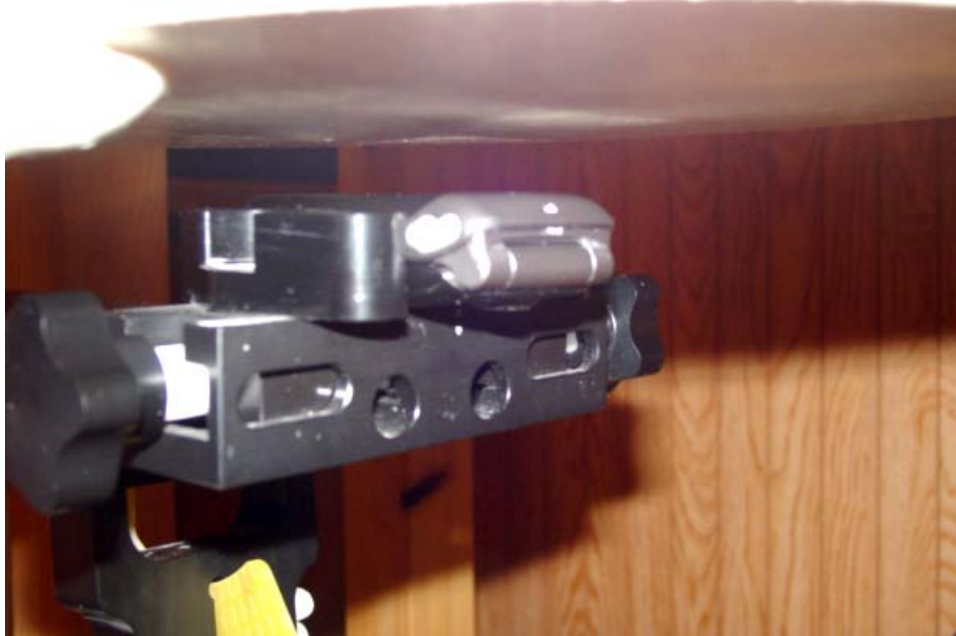
Figure 12.6 body SAR setup closed (with 15mm air separation)
