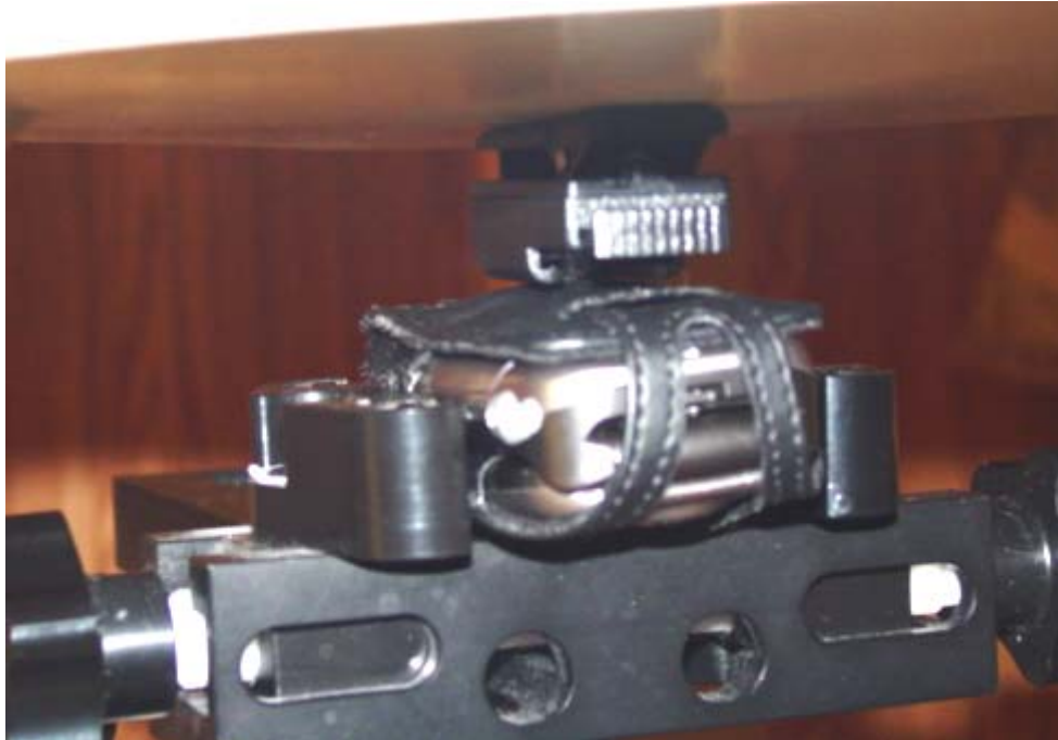
Figure 12.8 body SAR setup closed (with standard leather case)
