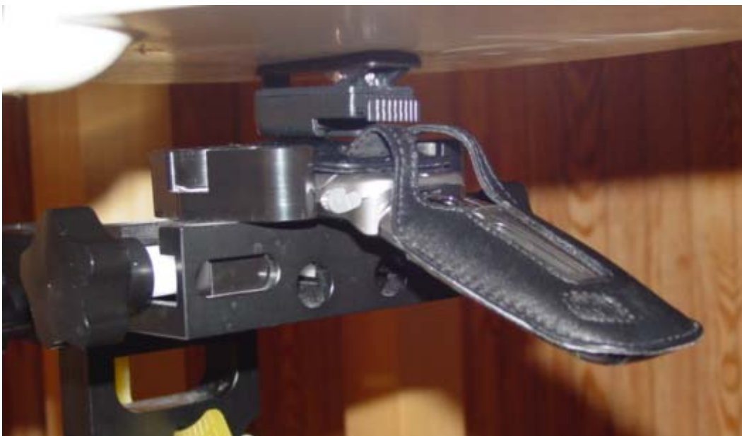
Figure 12.11 body SAR setup open (with premium leather case)
