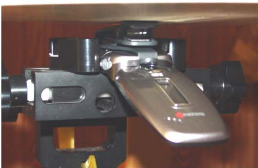
Figure 12.5 body SAR setup open (with holster)
