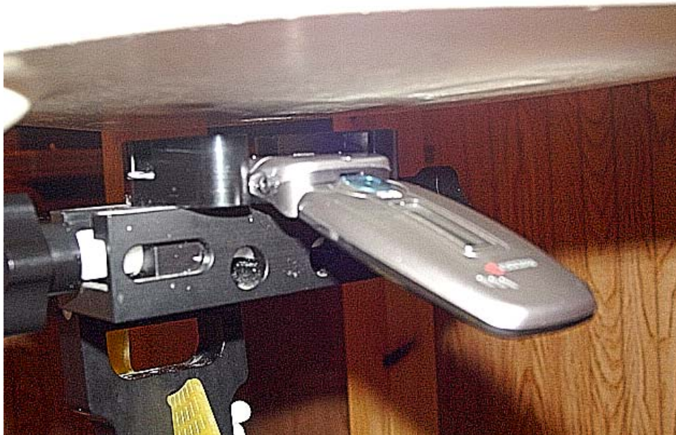
Figure 12.7 body SAR setup open (with 15mm air separation)
