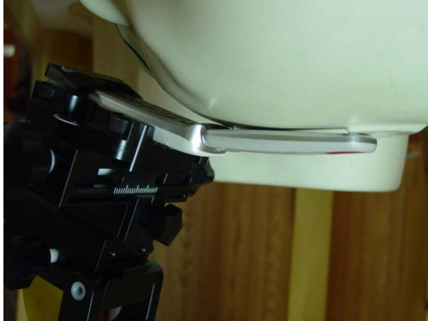
Phone against the head with standard battery (left cheek position)
