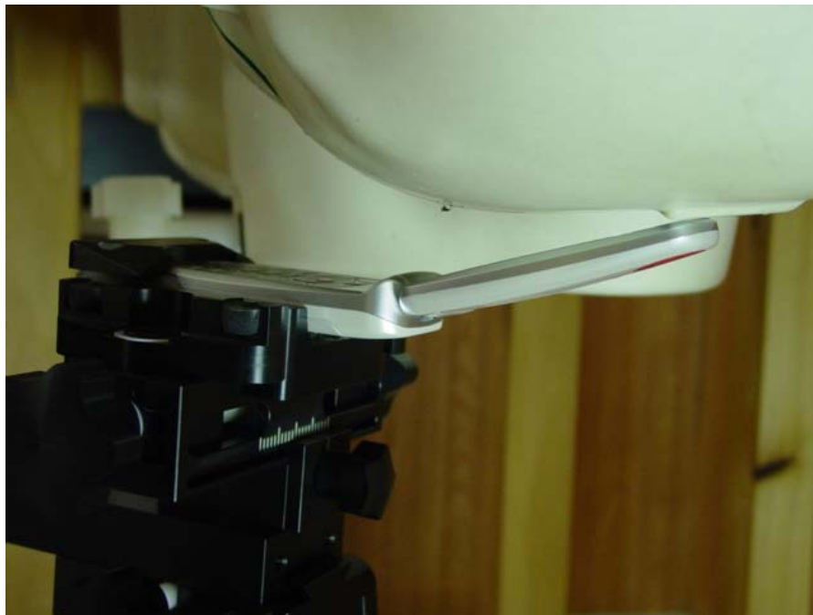
Phone against the head with standard battery (left tilt position)
