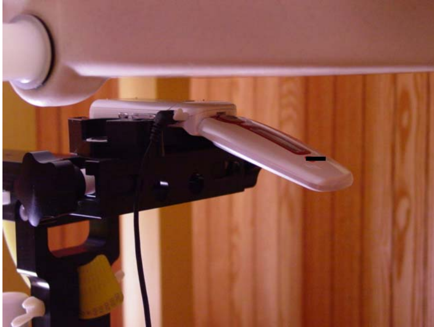
Body SAR setup with standard battery Open (with 12mm air gap)
