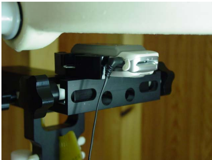
Body SAR setup with extended battery Closed (with 12mm air gap)
