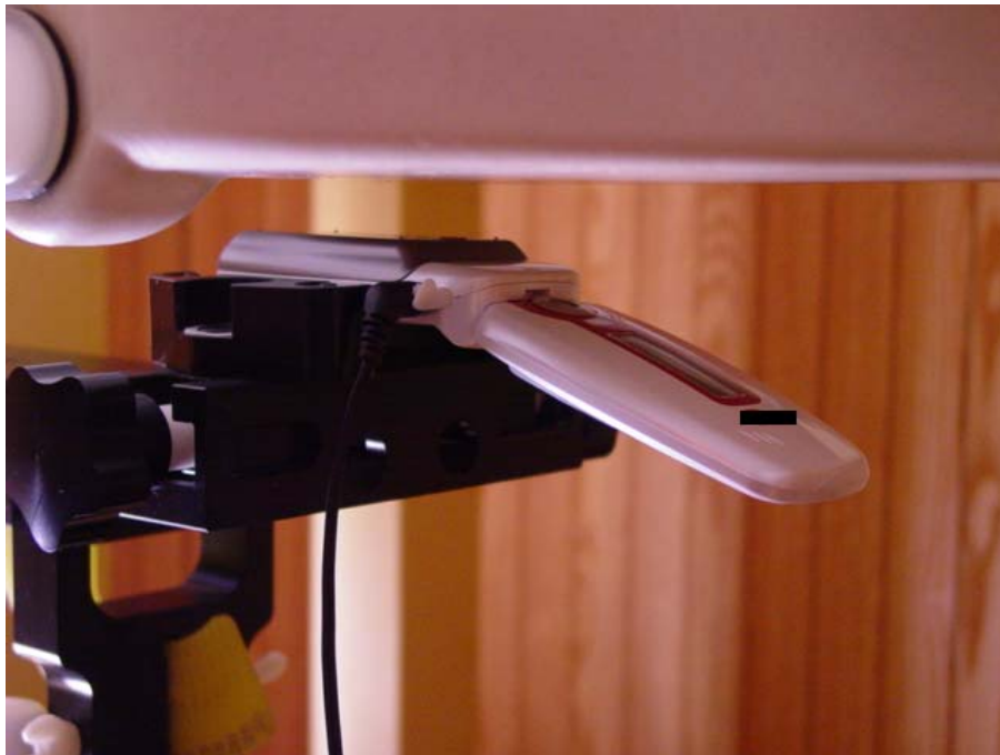
Body SAR setup with extended battery Open (with 12mm air gap)
