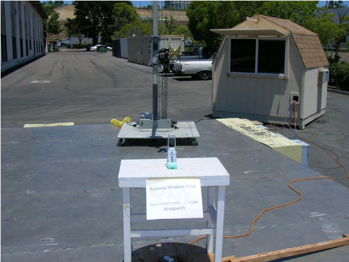
Figure 4. FCC, Part 24 Radiated Emissions Test Configuration
