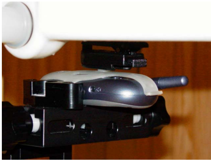
Figure 10.4 body sar setup (with Holster)
