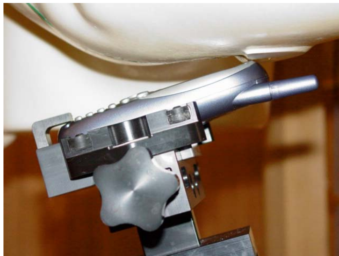
Figure 10.3 phone against the head (left tilt position)
