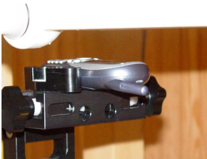
Figure 10.7 Face SAR setup (with 25mm air separation)
