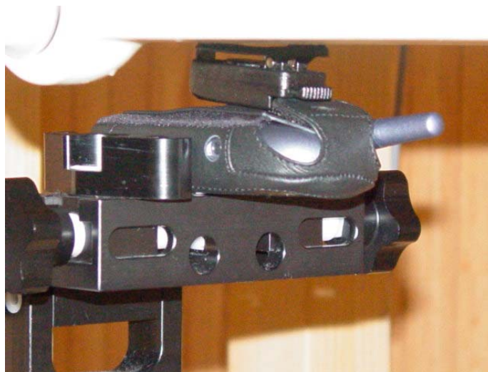
Figure 10.5 body sar setup (with leather case)
