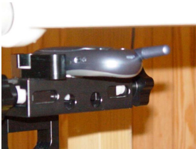
Figure 10.6 body sar setup (with 15mm air separation)
