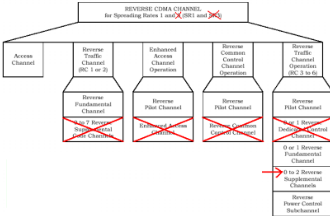
Figure 2.1.3.1.1-1. Reverse CDMA Channels Received at the Base Station
