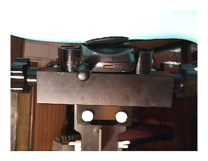
Test Setup for Body-worn SAR
