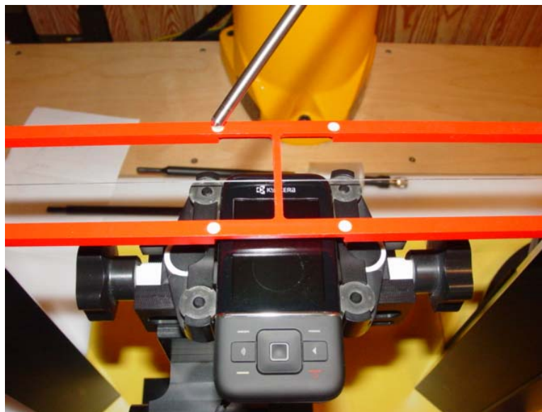
Figure 1b - HAC T-Coil Test Setup for Close Configuration
