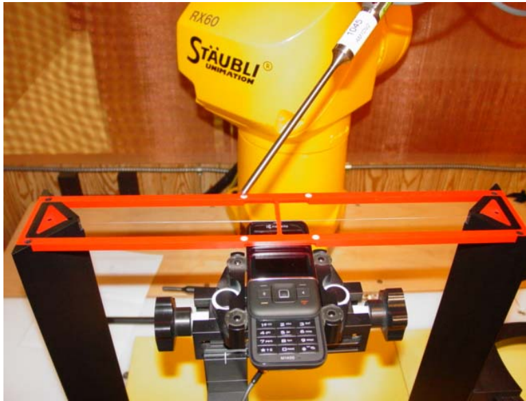
Figure 2a - HAC T-Coil Test Setup for Open Configuration
