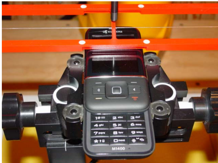
Figure 2b – HAC RF Emission Test Setup for Open Configuration
