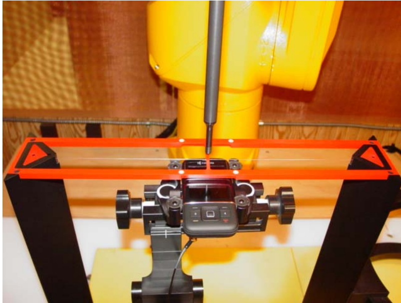
Figure 1a – HAC RF Emission Test Setup for Close Configuration
