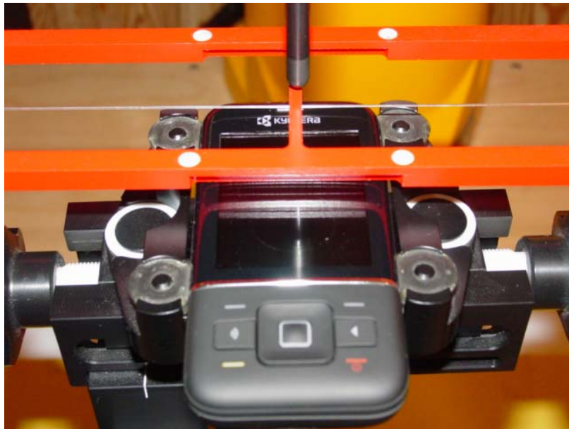
Figure 1b – HAC RF Emission Test Setup for Close Configuration
