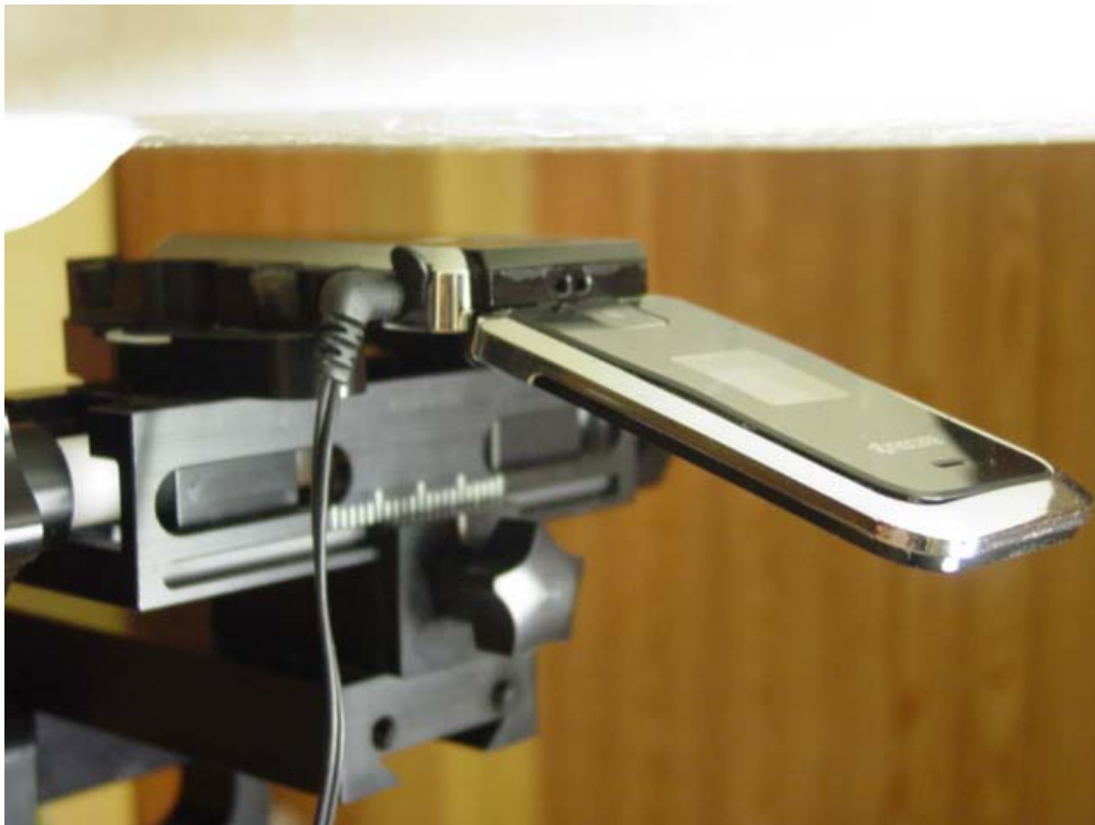
Figure 9E.4 Body SAR Phone Open setup (15mm Air Separation)
