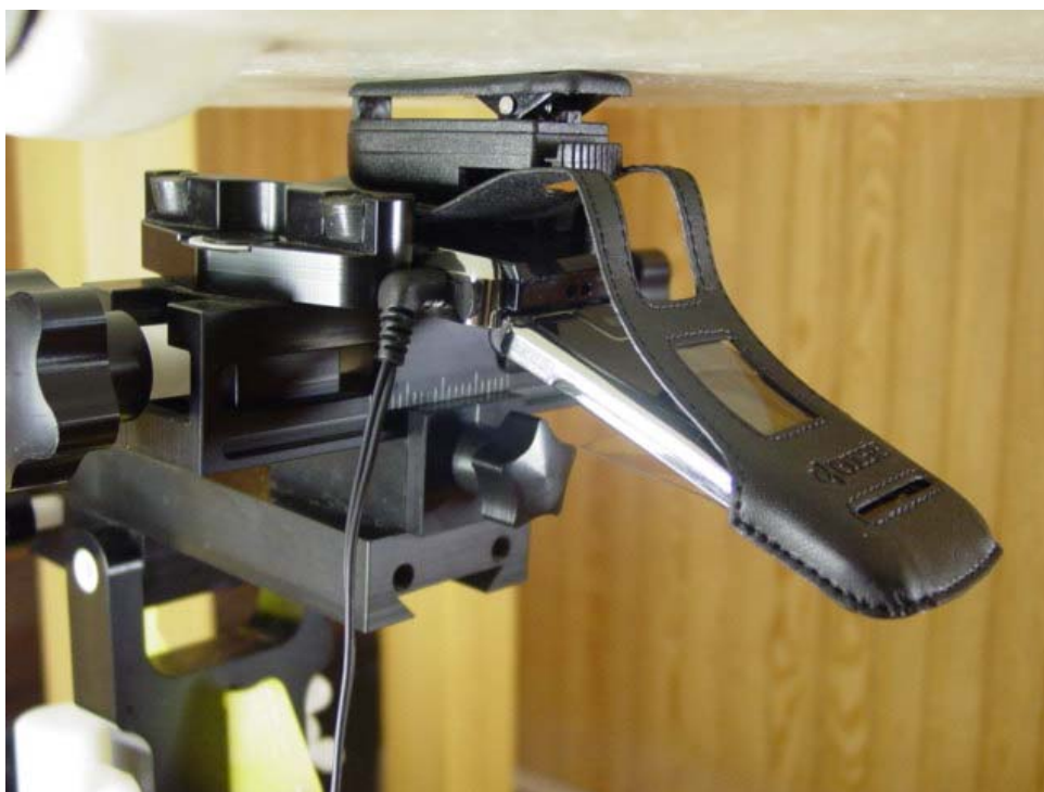
Figure 9E.8 Body SAR Phone Open setup (Leather Case)
