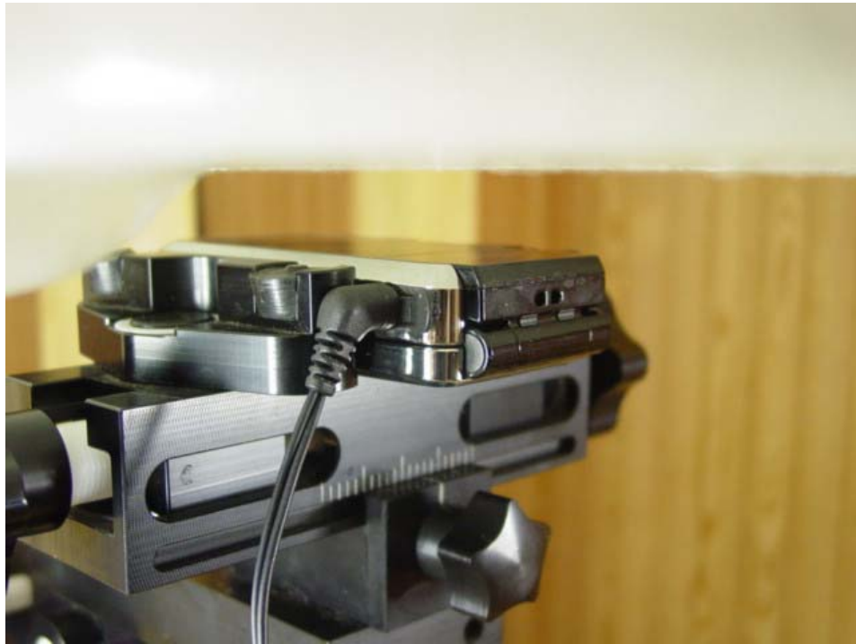
Figure 9E.3 Body SAR Phone Closed setup (15mm Air Separation)
