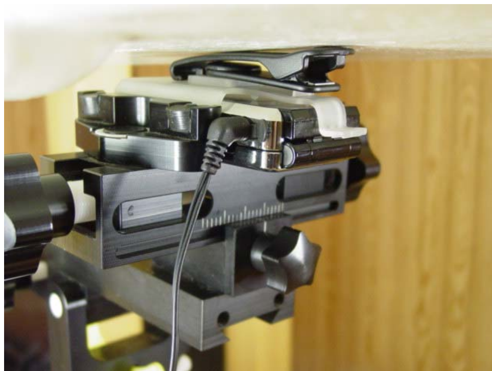
Figure 9E.6 Body SAR Phone Closed setup (Holster)
