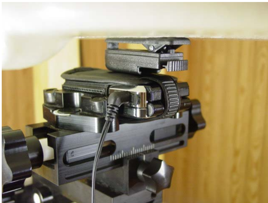
Figure 9E.5 Body SAR Phone Closed setup (CV90-61344-03)
