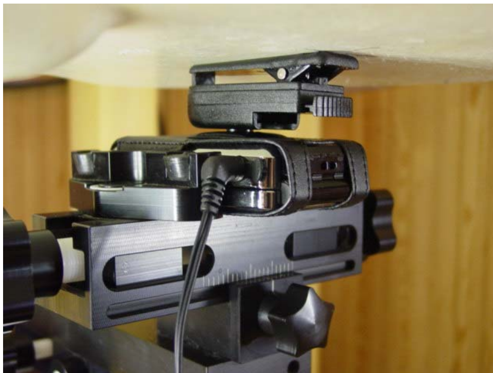
Figure 9E.7 Body SAR Phone Closed setup (Leather Case)
