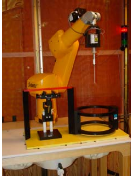
Figure 4.2a T-Coil setup with Helmholtz Coil
