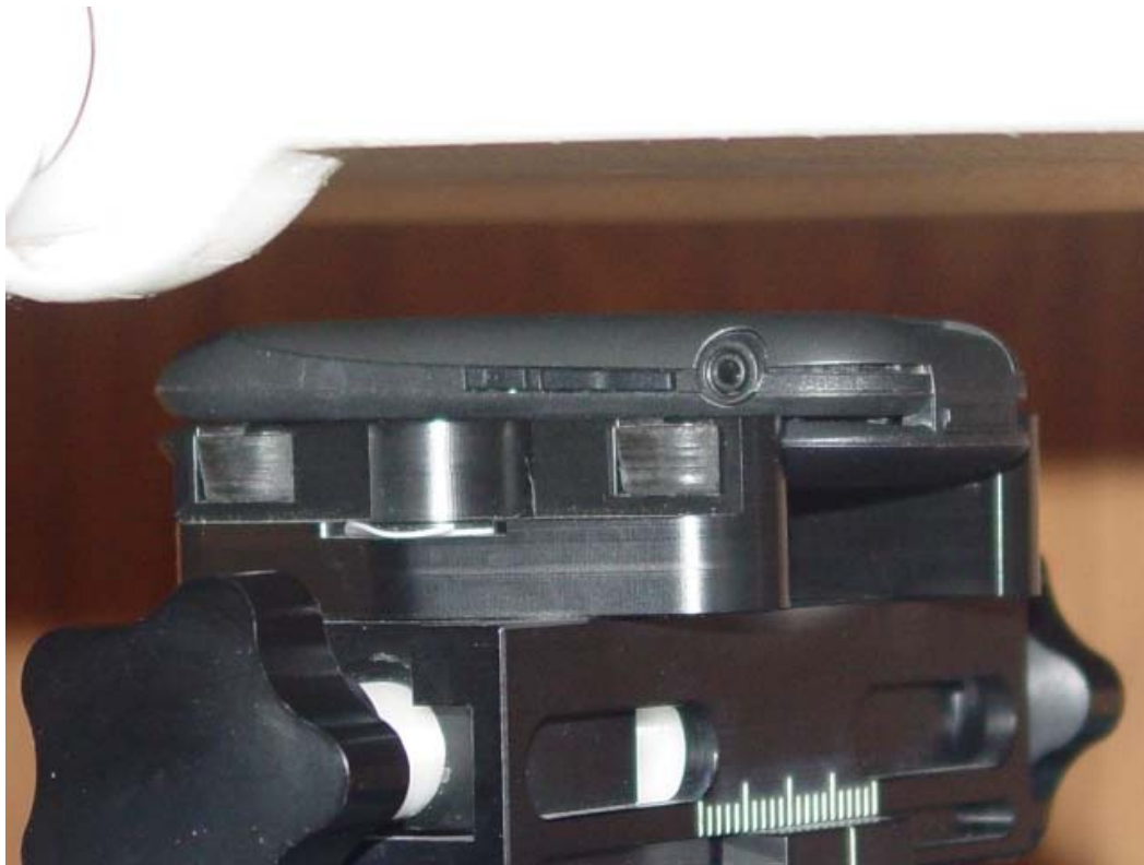
Figure 9E.4 Body SAR setup (Closed, Face Down, 15mm Air Separation)
