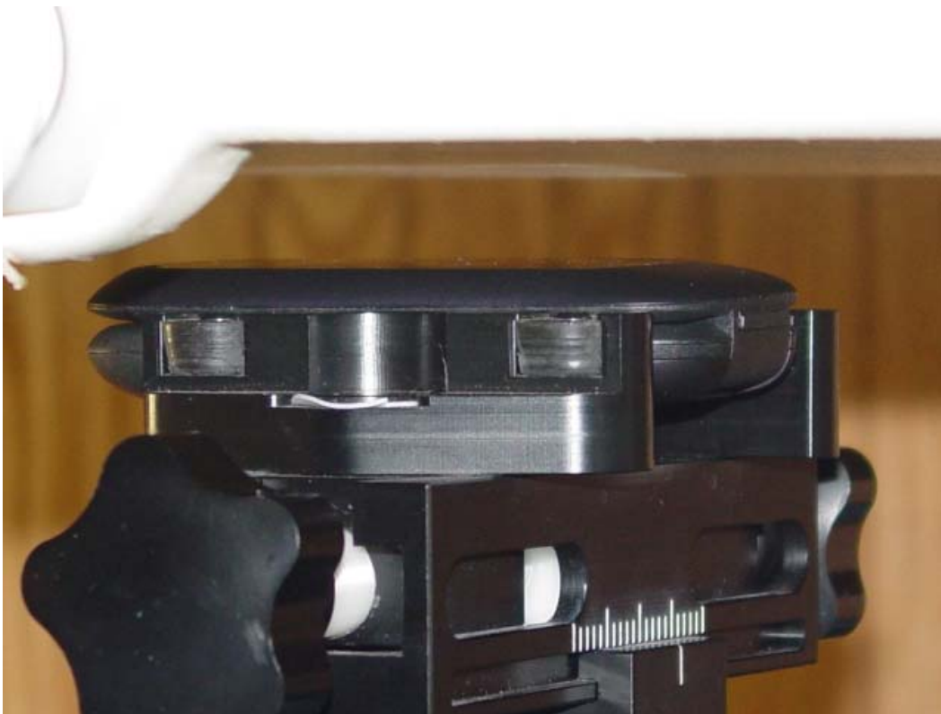
Figure 9E.5 Body SAR setup (Closed, Face Up, 15mm Air Separation)
