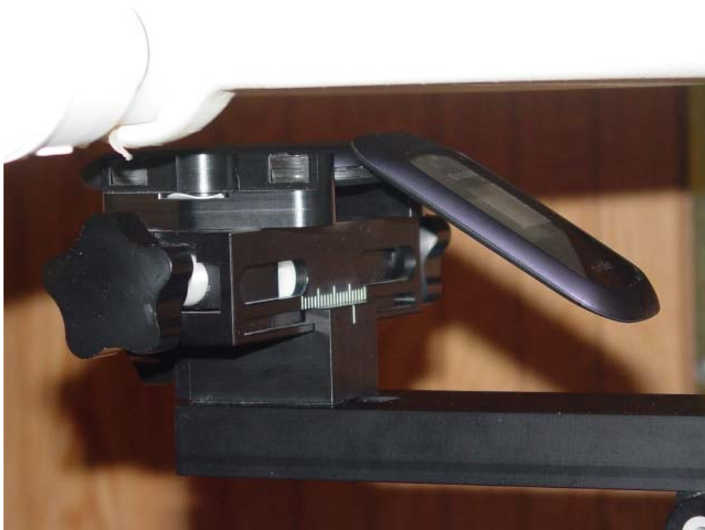
Figure 9E.6 Body SAR setup (Open, Face Down, 15mm Air Separation)
