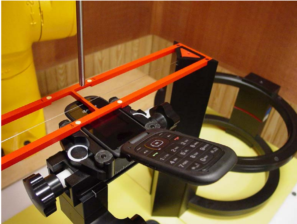
Figure 1a - HAC T-Coil Test Setup
