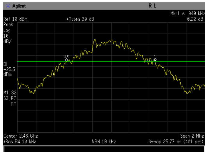
Figure 3-3a: 20dB Bandwidth basic rate, Channel 78.
