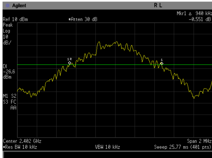
Figure 3-1a: 20dB Bandwidth basic rate, Channel 0.
