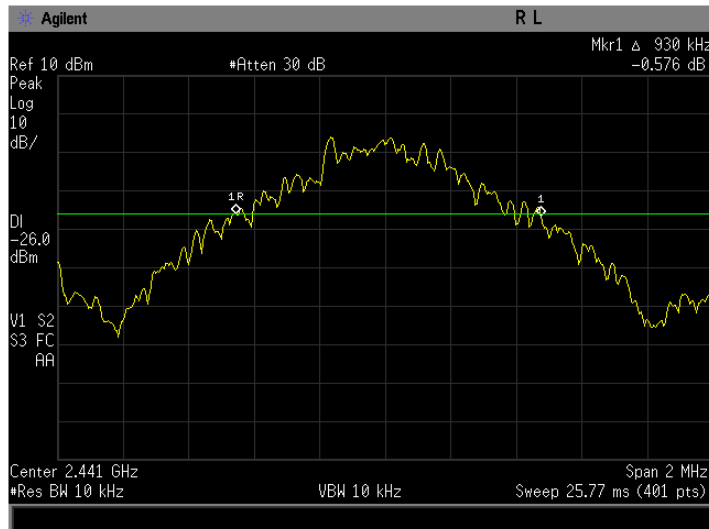
Figure 3-2a: 20dB Bandwidth basic rate, Channel 39.
