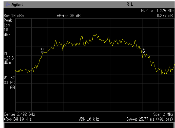
Figure 3-1b: 20dB Bandwidth EDR 2Mbps, Channel 0.
