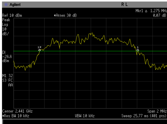
Figure 3-2b: 20dB Bandwidth EDR 2Mbps, Channel 39.
