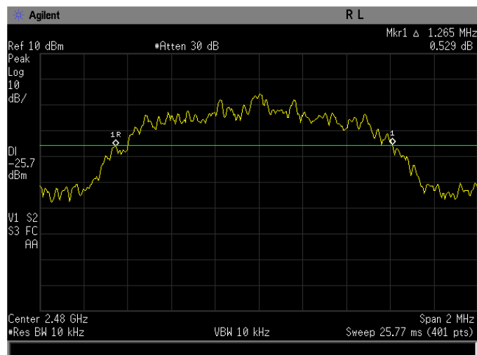
Figure 3-3c: 20dB Bandwidth EDR 3Mbps, Channel 78.
