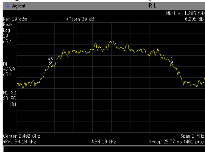
Figure 3-1c: 20dB Bandwidth EDR 3Mbps, Channel 0.
