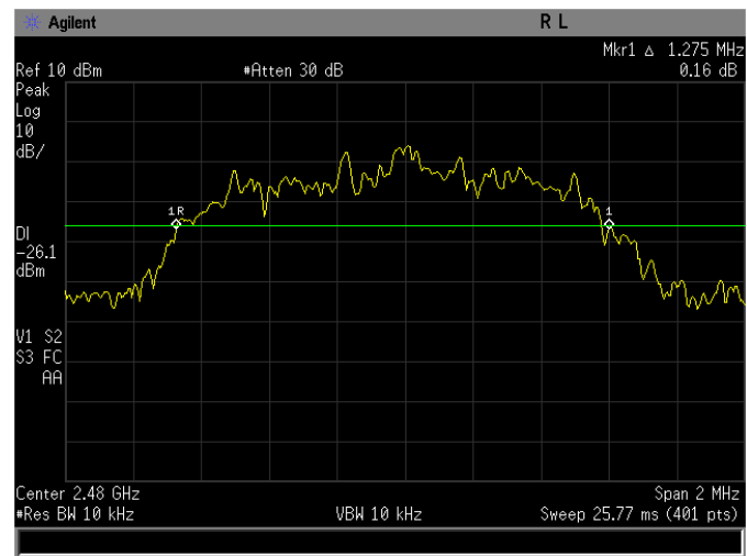
Figure 3-3b: 20dB Bandwidth EDR 2Mbps, Channel 78.
