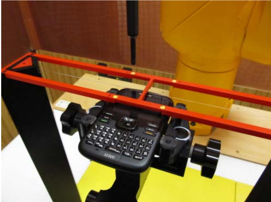
Figure 1a – HAC RF Emission Test Setup
