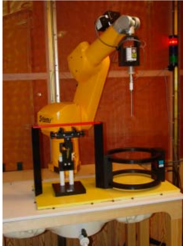
Figure 5.2a T-Coil setup with Helmholtz Coil
