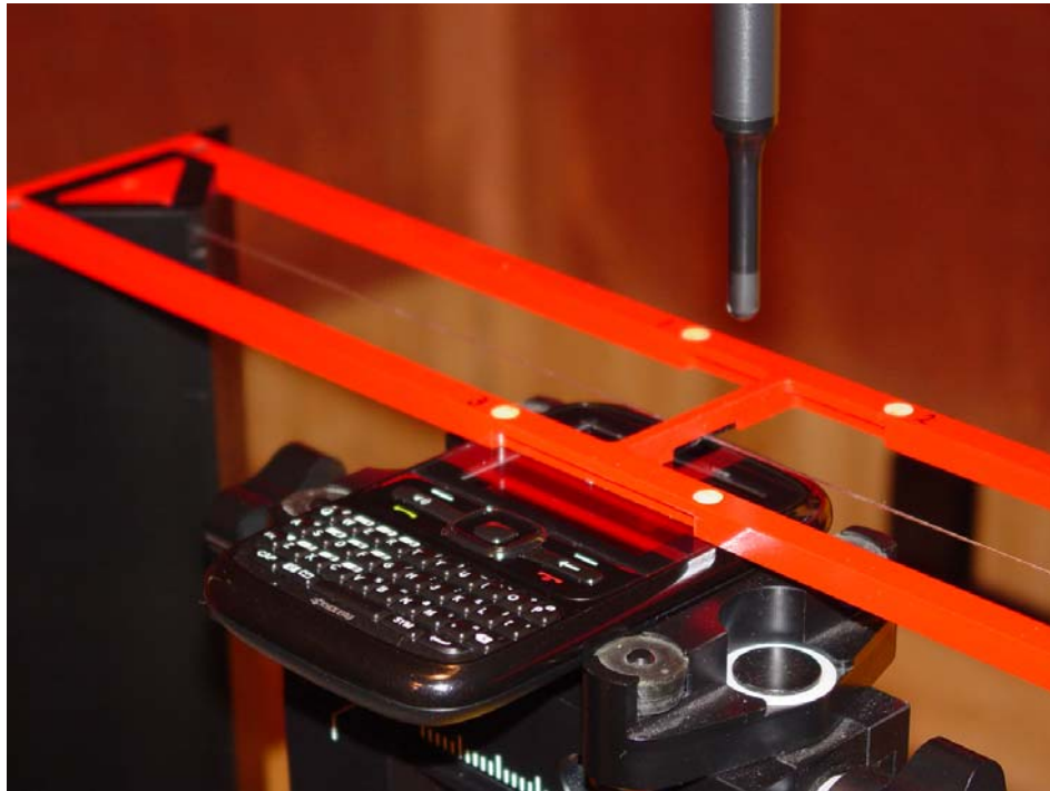
Figure 1a – HAC-RF Test Setup
