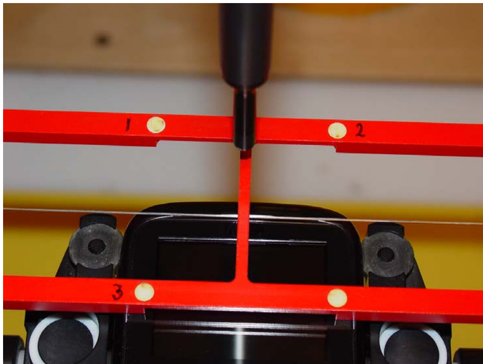
Figure 1b – HAC-RF Test Setup
