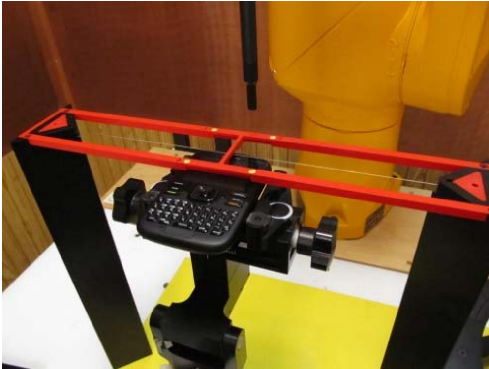
Figure 1a – HAC RF Emission Test Setup
