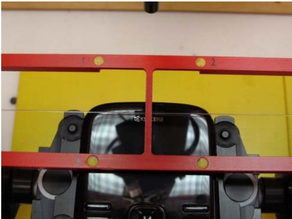
Figure 1b – HAC RF Emission Test Setup
