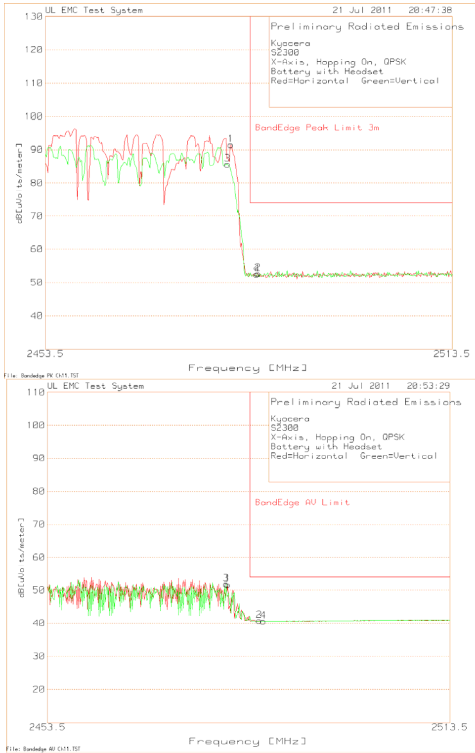
Figure 13 Radiated Emissions Graph Hi Channel DH5 QPSK Bandedge
