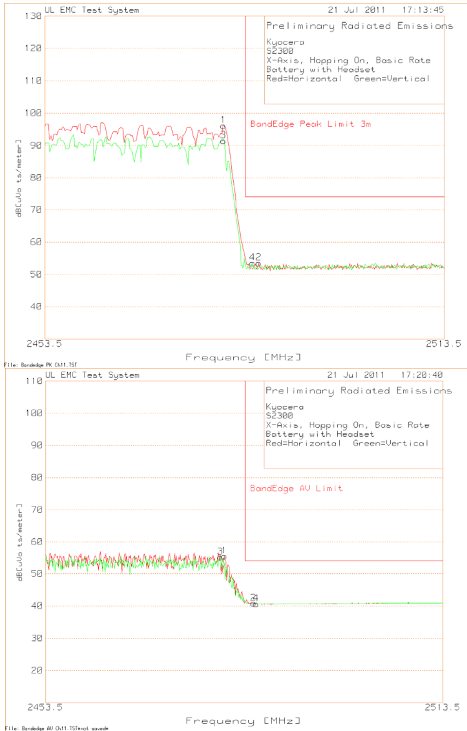
Figure 11 Radiated Emissions Graph Hi Channel DH5 Bandedge
