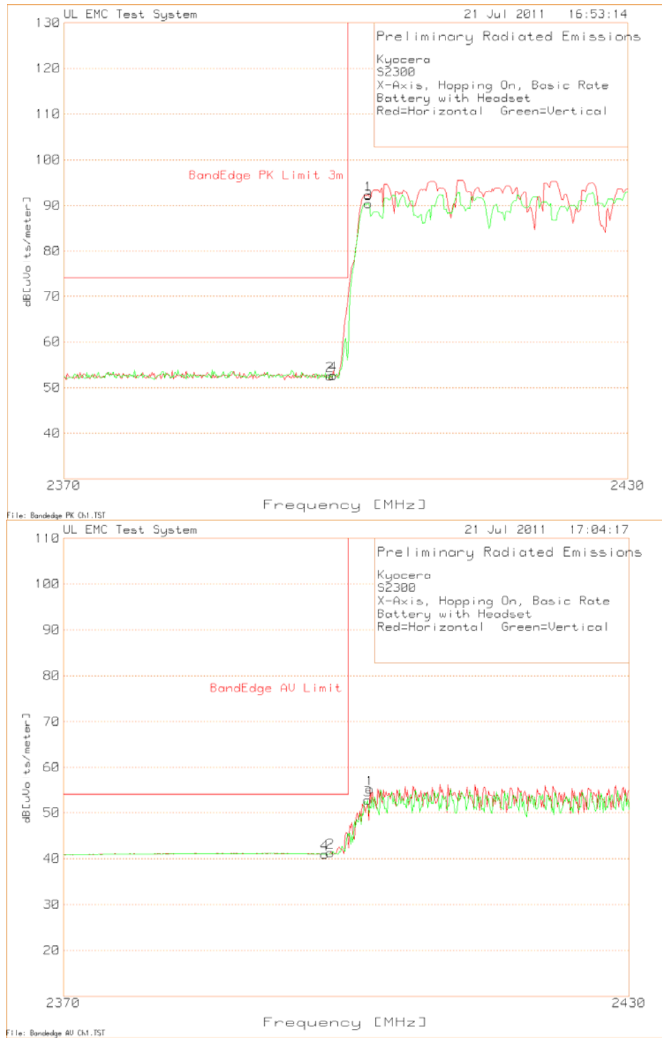
Figure 10 Radiated Emissions Graph Low Channel DH5 Bandedge
