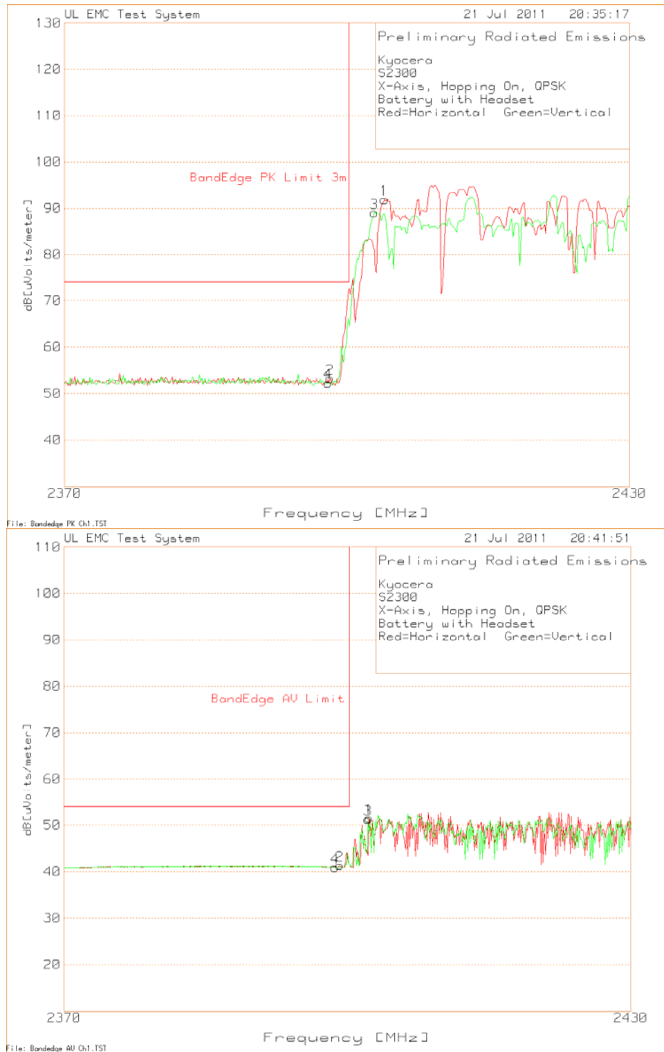
Figure 12 Radiated Emissions Graph Low Channel DH5 QPSK Bandedge
