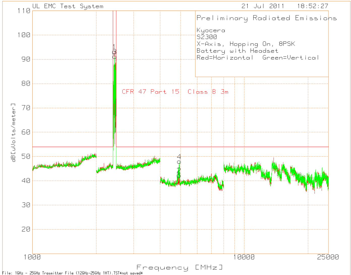
Figure 9 Radiated Emissions Graph Hopping 8PSK DH5
